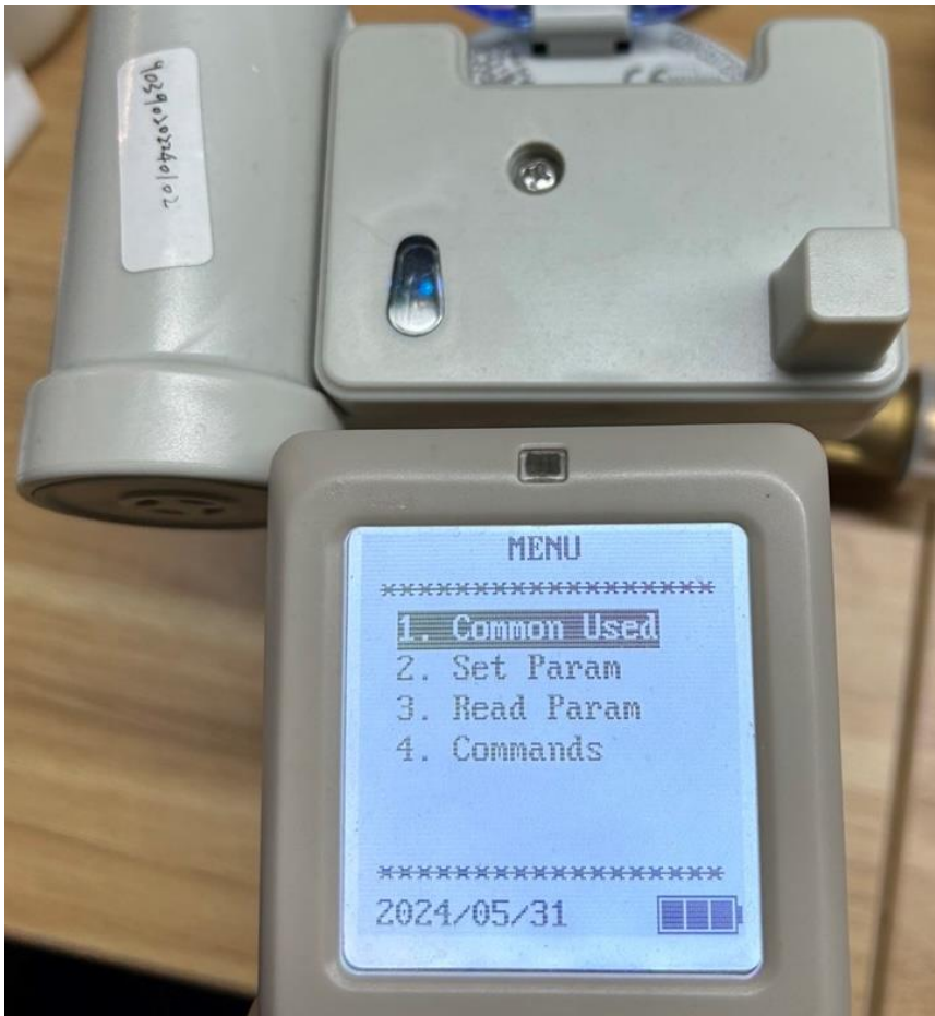
Figure 7: Configuring the MIU with the Handheld Device
