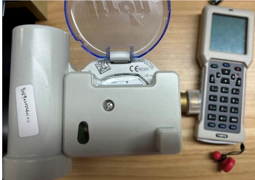
Figure 5: To wake up the MIU with a magnet
