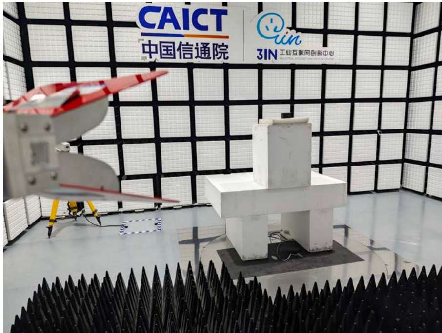
Description: Back view of Radiated Emission Test Setup (1GHz -18GHz) WIFI Test
