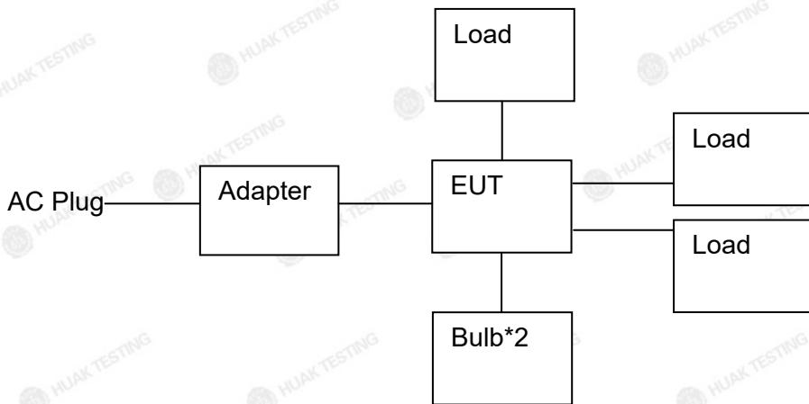
Operation of EUT during radiation below 1GHz testing:
