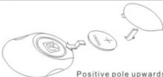
Positive pole upwards to install the battery.
