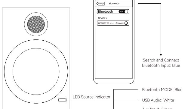
1. The speaker defaults to Bluetooth mode for the initial starting up. In non-Bluetooth mode, short press "PAIR" button on the back of the speaker, activate your device's Bluetooth and search for "HOTMAY BS Mini" and select. When the speaker is in Bluetooth pairing status, the blue light will keep flashing. When the speaker is connected to a device, the blue light will be constantly on.
