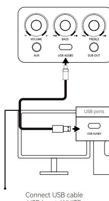
After the speaker is turned on, short press Mode control button on the back of the speaker. In USB audio mode, white light will be constantly on. Connect the USB cable to computer, go to computer's setting, select "HOTMAY BS Mini".
