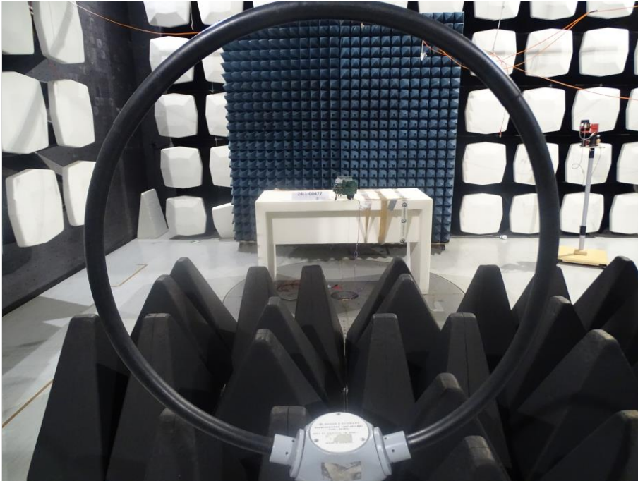
Photograph 11: EUT test setup in the semi anechoic chamber, overview_EUT elevation 90°
