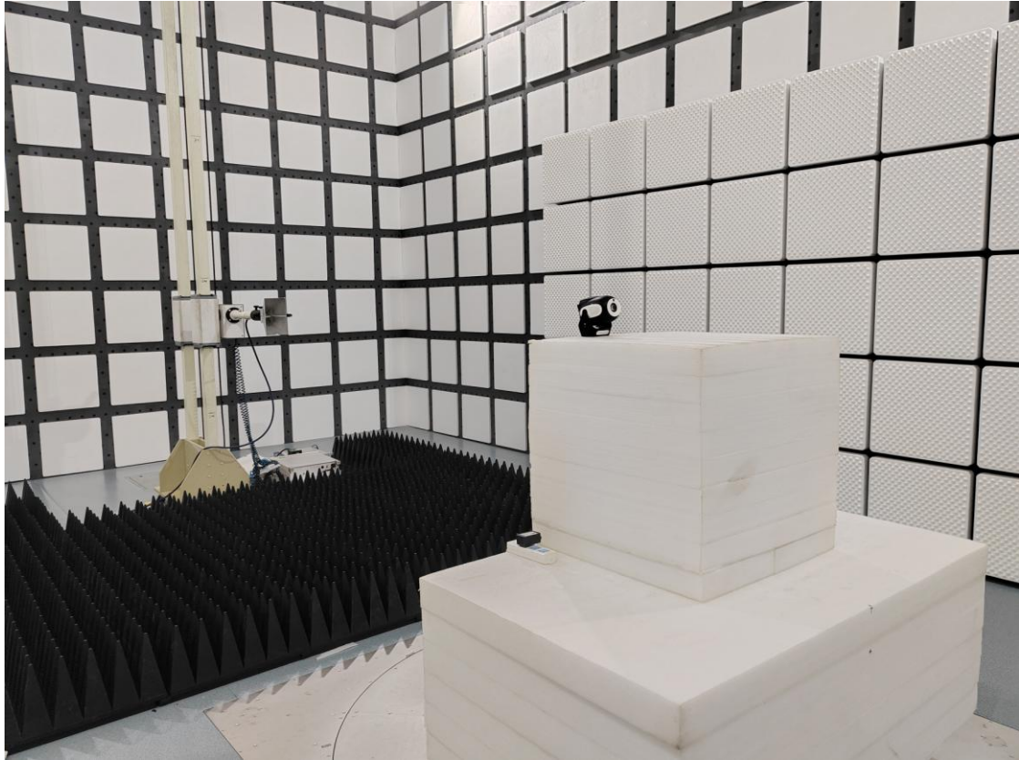
Radiated Spurious Emissions Test View (1GHz-18GHz)
