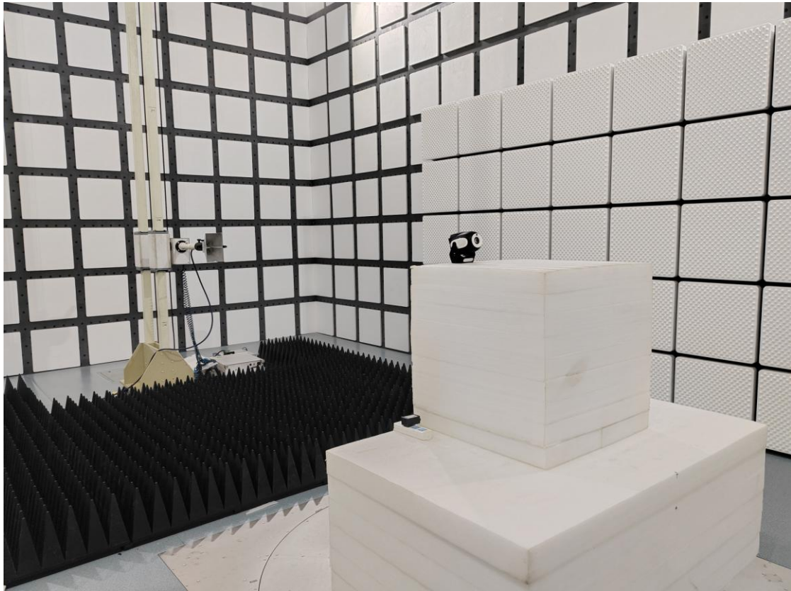
Radiated Spurious Emissions Test View (1GHz-18GHz)
