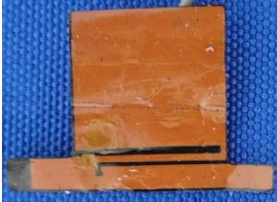
A photograph of the antenna, which is a rectangular FPCB (Flexible Printed Circuit Board) with a central orange square and two black rectangular components attached to the bottom edge. It is placed on a blue textured surface. |                   |
