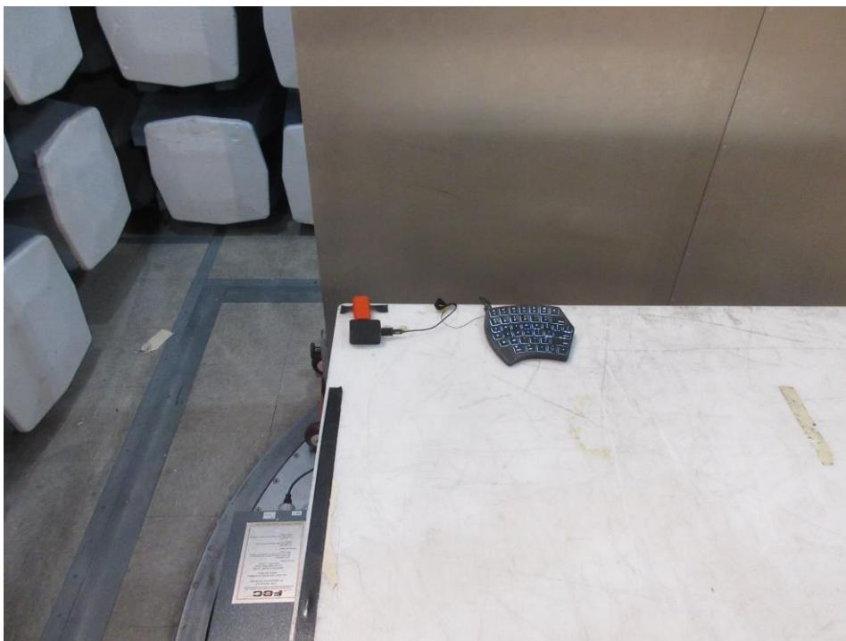
**1.8. AC Line Conducted Test: Side View**
