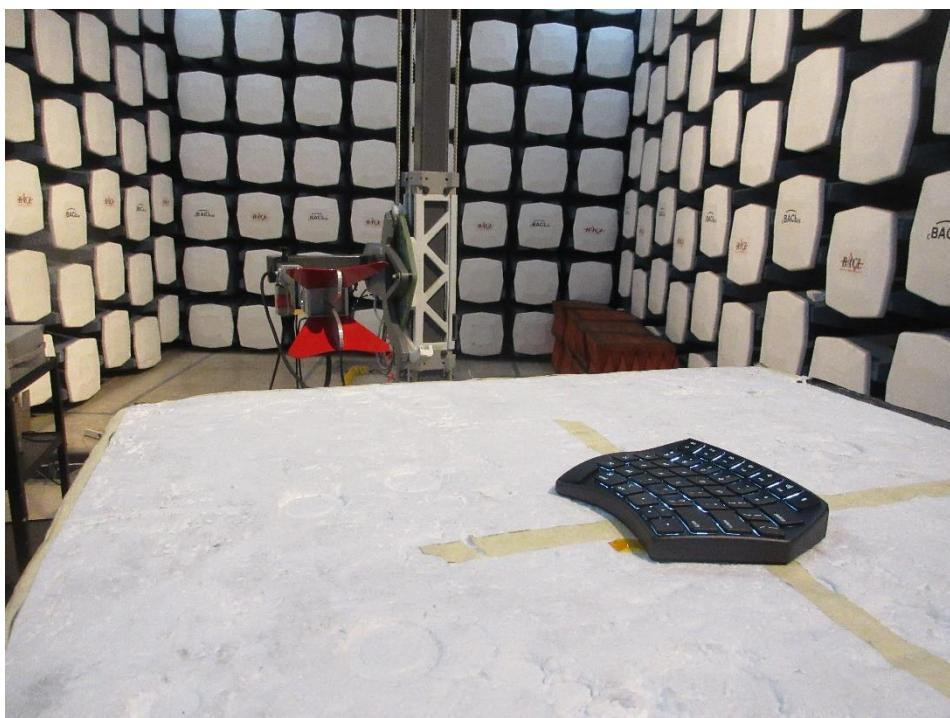
**1.5. Radiated 18 – 26.5 GHz: Front View**
