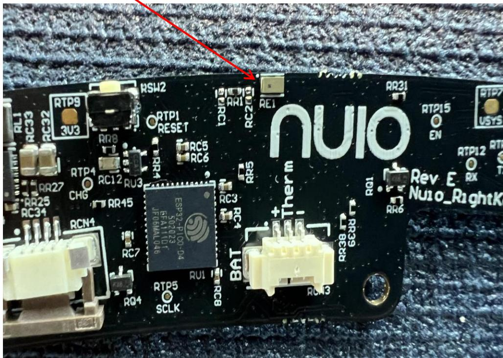
**1.7 EUT (Right) – ISM Antenna**
