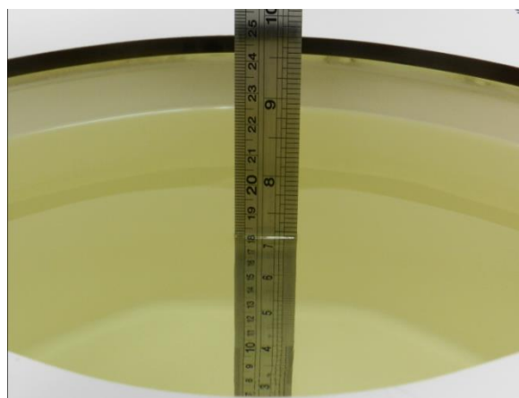
Fig 10.2 Photo of Liquid Height for Body SAR
