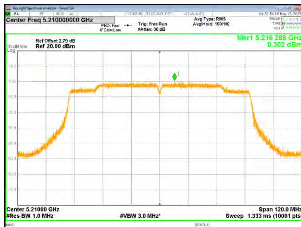
(802.11ac80) PSD plot on channel 42
