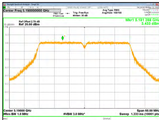
(802.11n40) PSD plot on channel 38
