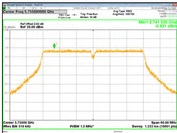
(802.11ac40) PSD plot on channel 159
