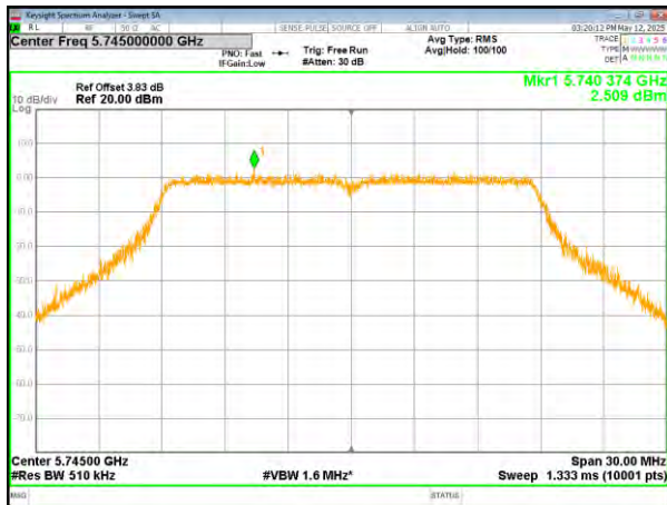
(802.11ac20) PSD plot on channel 157
