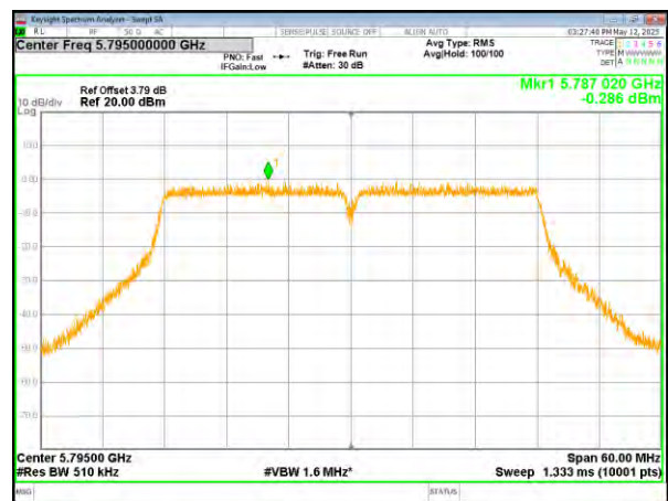
(802.11n40) PSD plot on channel 159
