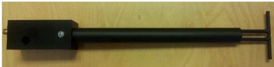
Figure 1 – MVG COMOSAR Validation Dipole
