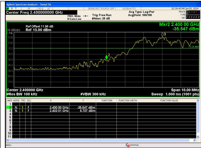
Out Of Band Emission(Left) 8DPSK_3-DH5_Channel Hopping
