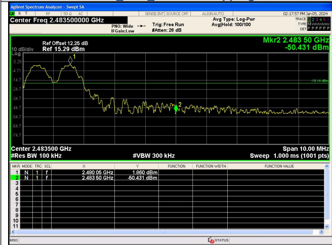
Out Of Band Emission(Right) GFSK_DH5_Channel Hopping
