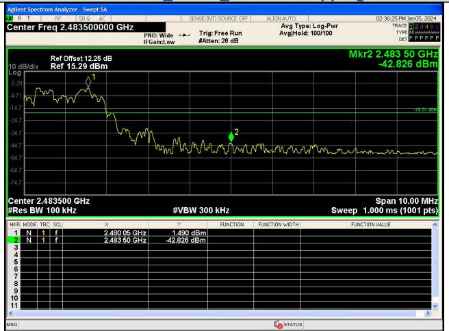
Out Of Band Emission(Right) \pi/4 DQPSK_2-DH5_Channel Hopping
