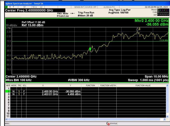
Out Of Band Emission(Left) 8DPSK_3-DH5_Channel Hopping
