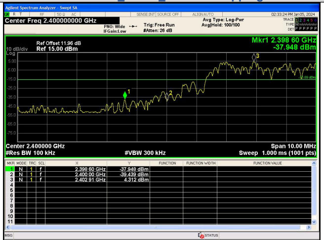
Out Of Band Emission(Left) \pi/4 DQPSK_2-DH5_Channel Hopping
