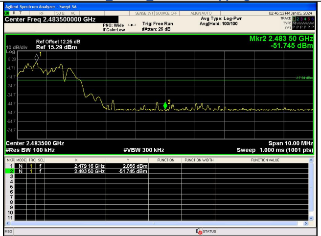
Out Of Band Emission(Right) 8DPSK_3-DH5_Channel Hopping
