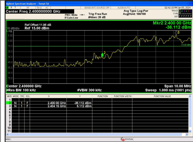
Out Of Band Emission(Left) 8DPSK_3-DH5_Channel Hopping
