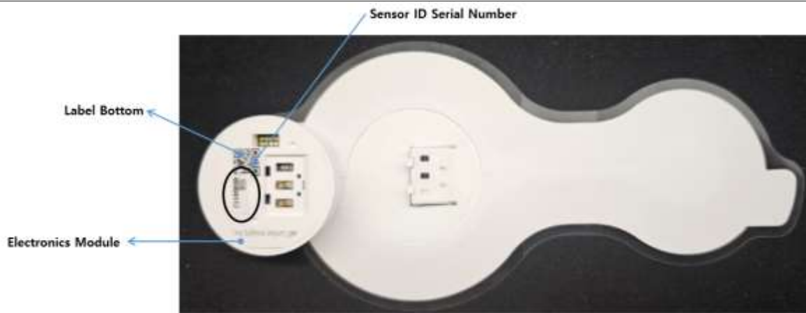
Figure 3.8. The exposed Electronics Module following removal of the foam cover. The barcode uses the GS1 standard format.
