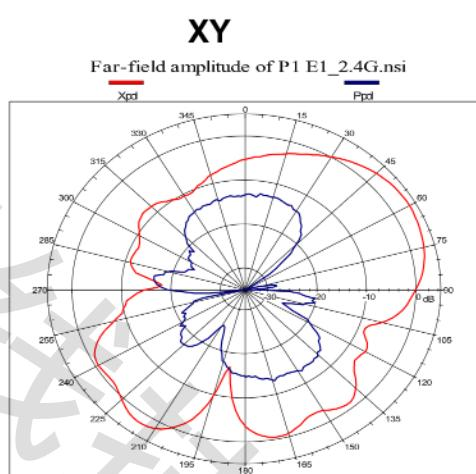
Source signal: Linearly polarized signal  $f_0 = 2450$  MHz
