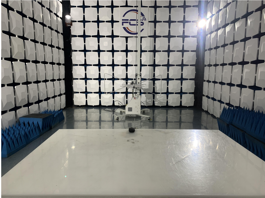
Above 1GHz for radiated emission test setup
