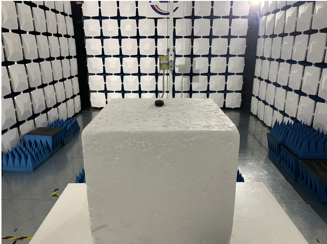
Above 1GHz for radiated emission test setup
