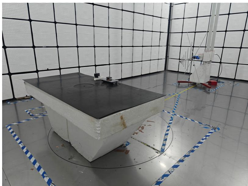
For 3m Radiated Emission 9 kHz - 30 MHz
