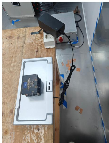
For 3m Radiated Emission 30 MHz - 1 GHz
