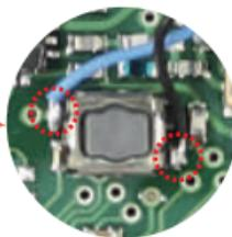
\*Weld the function line to the two diagonally opposite pins of the corresponding button, without distinguishing between positive and negative
