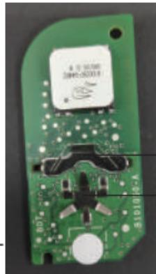
**Step 2: Take out the dedicated wiring harness from the accessory package, and according to the definition, group and weld the wiring harness to the corresponding key pins and battery holder positive and negative poles of the original car key circuit board**
