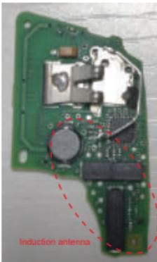
\*There are two common types of original car key induction antennas: a single 3D induction antenna or multiple single axis induction antennas, as shown in the left figure
