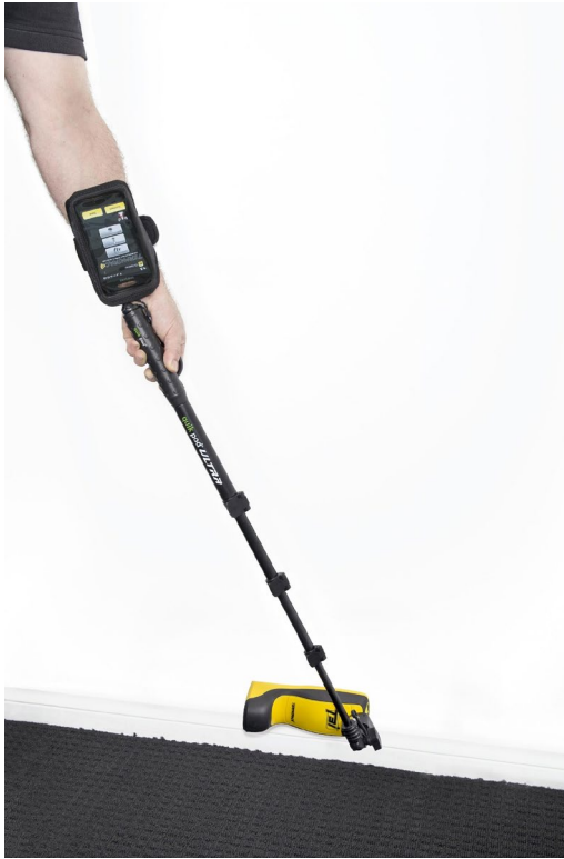
Figure 7 Monopod held to Skirting Board - Moisture Sensor
