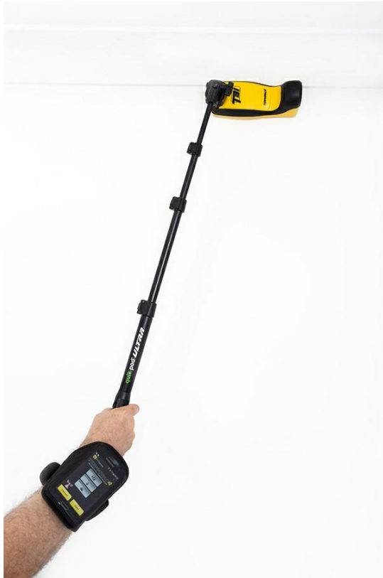
Figure 6 Monopod held to Ceiling - Moisture Sensor
