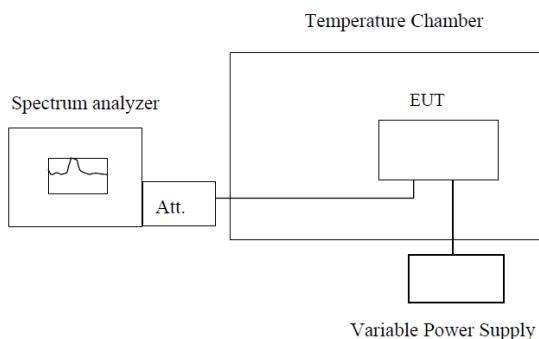
**Note :** Measurement setup for testing on Antenna connector
