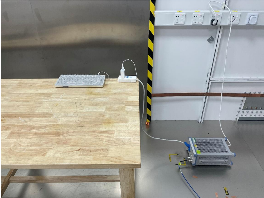
AC Power Line Conducted Emission
