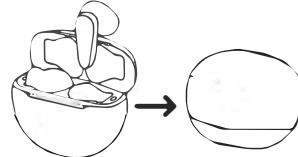
Put the earphone back into the charging compartment and close the cover, it will automatically shut down and charge. The charging compartment on the box, at this time, the display of the charging box lights up. Display battery
