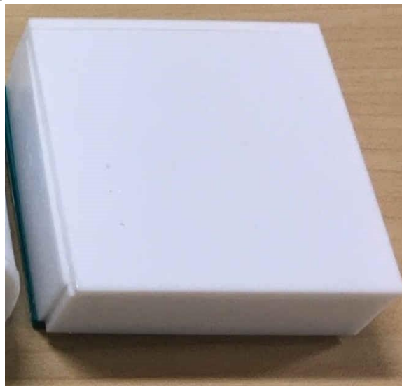
Figure 6-4. PTFE-Based Rectangular Radome With 1.524 mm Wall Thickness
