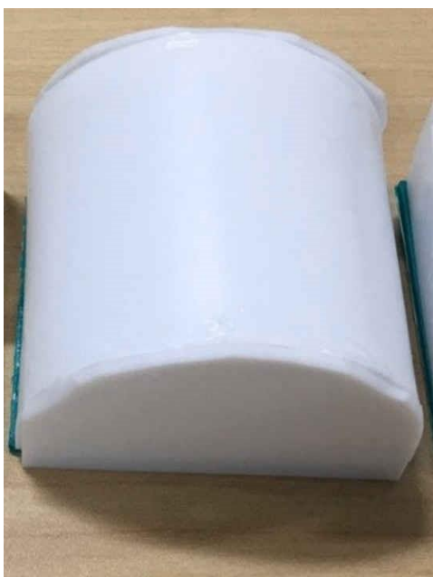
Figure 6-7. The PTFE Curved Shaped Radome With 1.524 mm Wall Thickness
