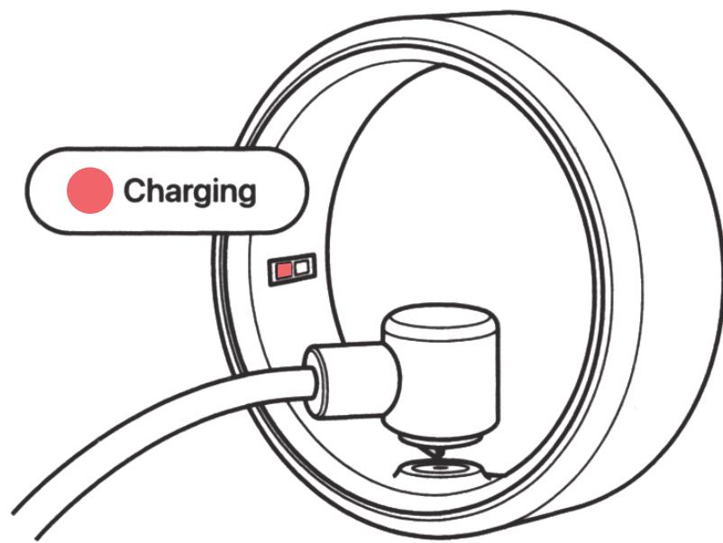
4. A flashing red light indicates that the ring is charging.
