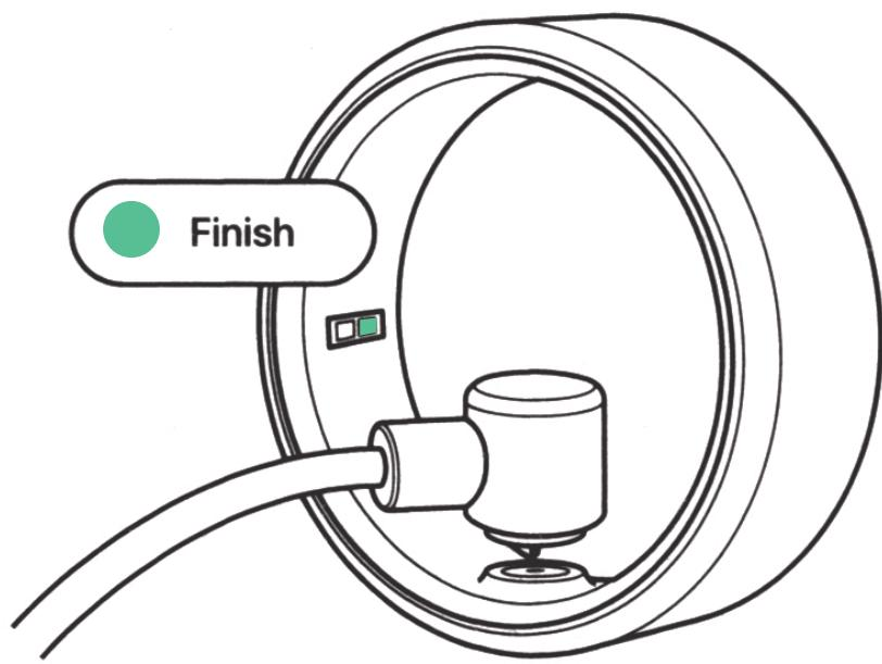
5. A flashing green light indicates that the ring has finished charging.
