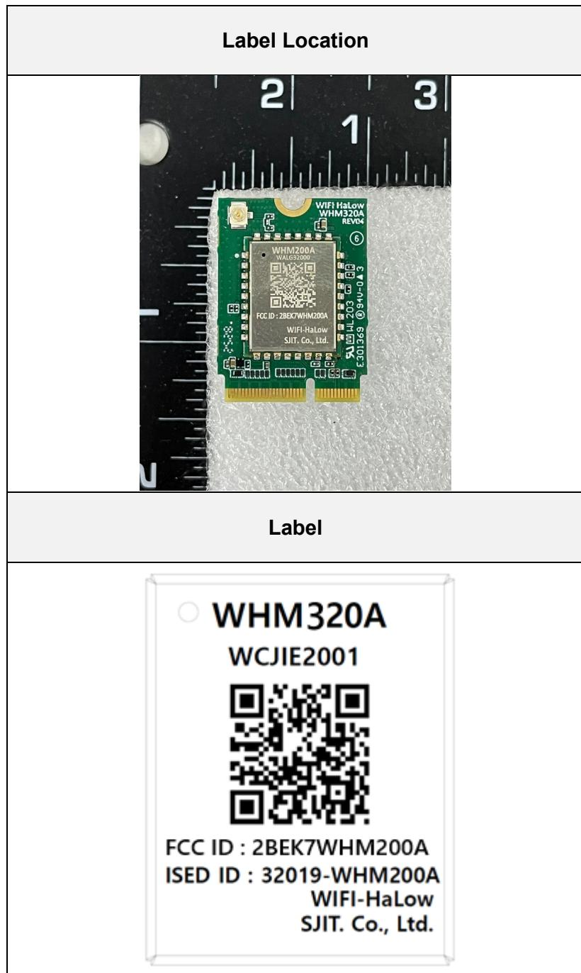
The device is so small that it is not practicable to place the statement specified under 15.19 statement request, the information required by this paragraph shall be placed in a prominent location in the User's Manual.
