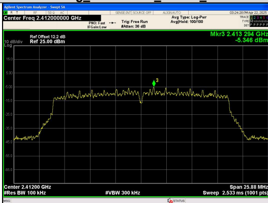
In-Band Reference Level IEEE 802.11n_Channel 1_20MHz_Antenna 0
