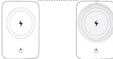
Ensure that the charging position is aligned with the wireless charger.
