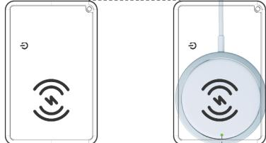
Ensure that the charging position is aligned with the wireless charger
