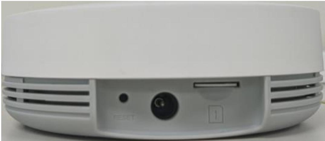
1. Insert the provided USIM into the Usim connector in the correct direction.
