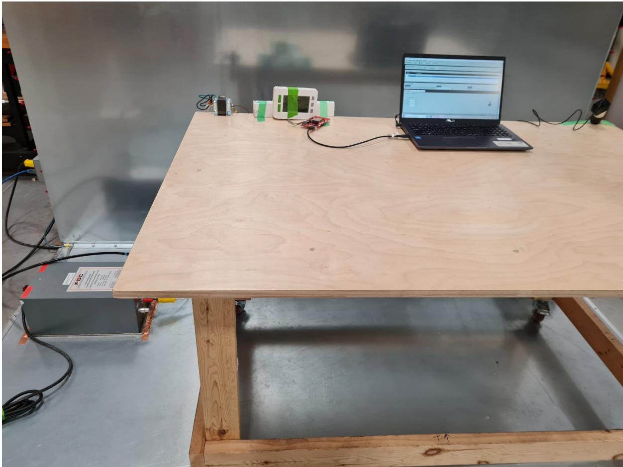
Figure 7 – Conducted Emissions Setup
