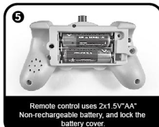
Remote control uses 2x1.5V "AA" Non-rechargeable battery, and lock the battery cover.
