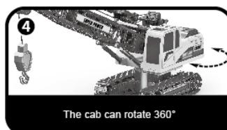
The cab can rotate 360°
