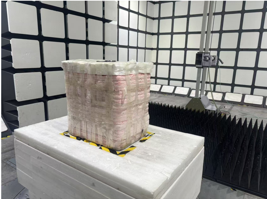
Radiated Emissions View (1-18 GHz)
