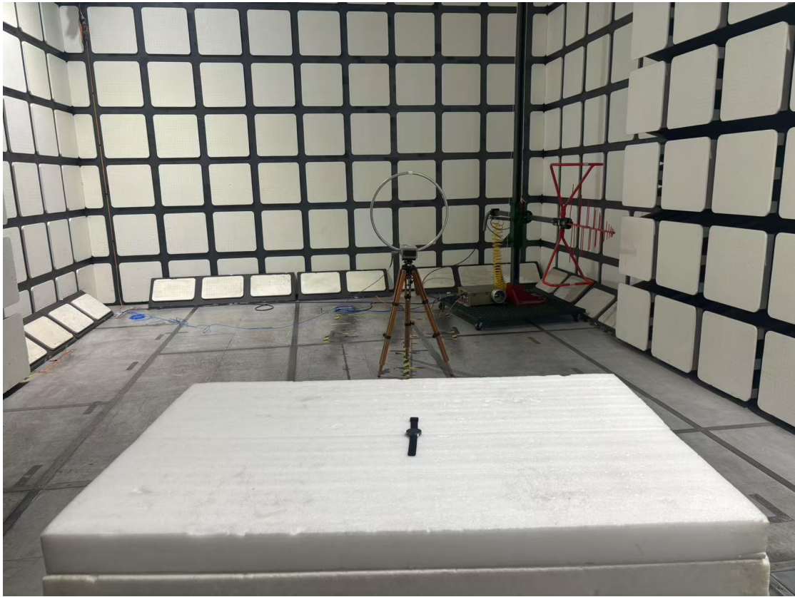
Radiated Emissions View (9 kHz- 30MHz)
