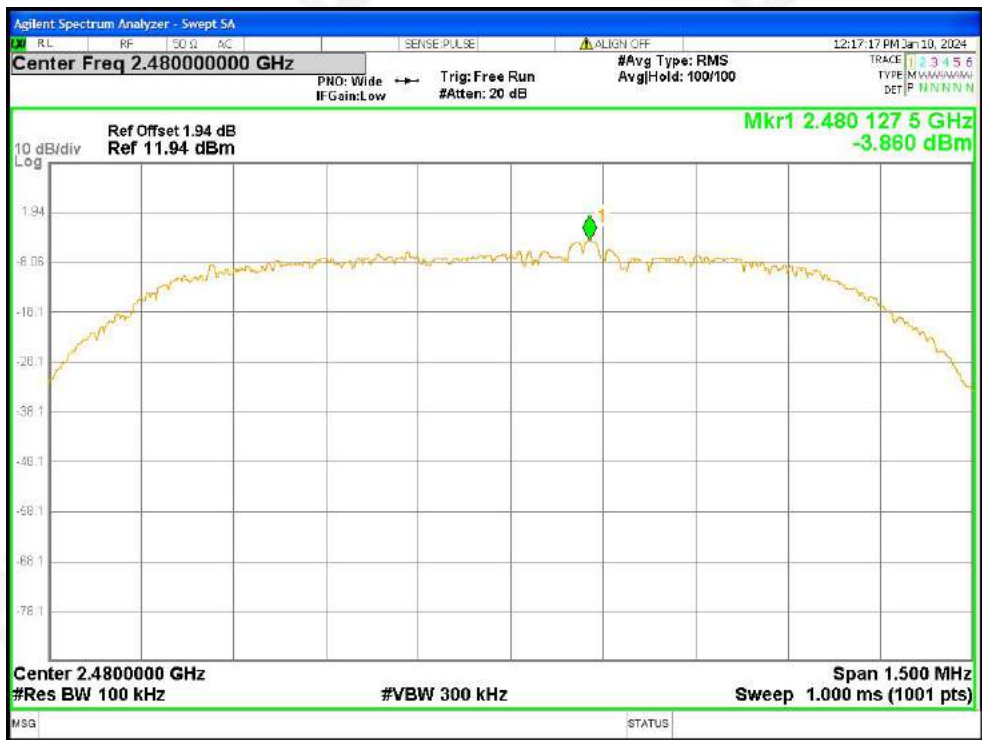
Tx. Spurious NVNT 3-DH5 2480MHz Ant1 Ref
