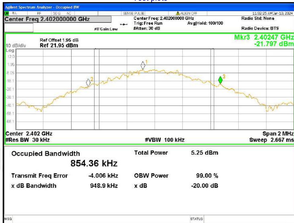
-20dB Bandwidth NVNT 1-DH5 2402MHz Ant1
