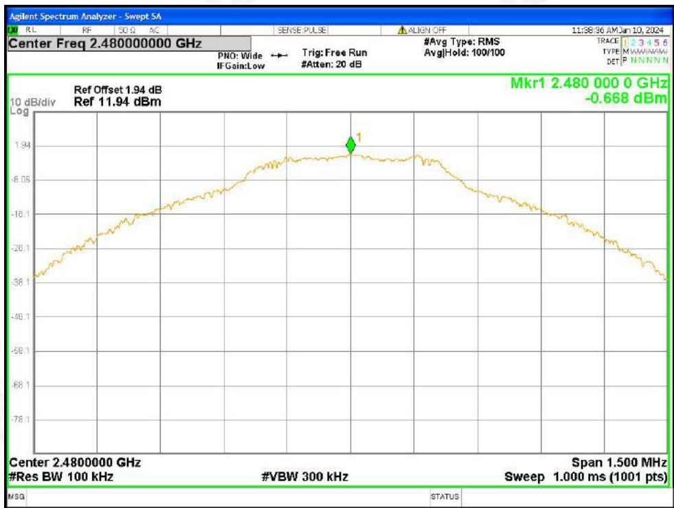
Tx. Spurious NVNT 1-DH5 2480MHz Ant1 Ref
