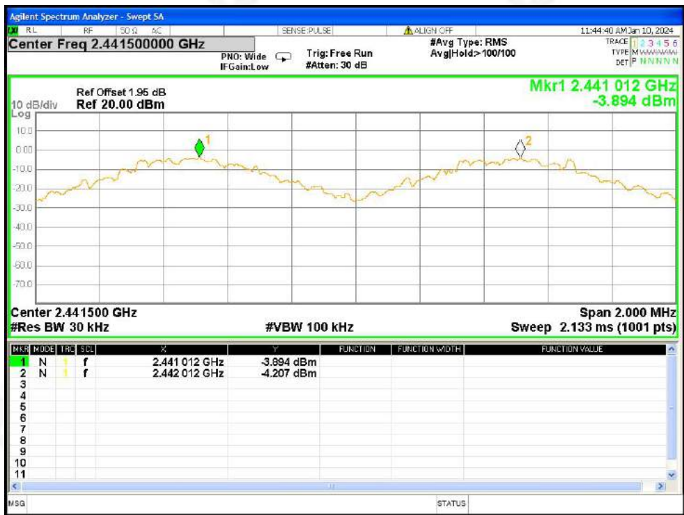
CFS NVNT 1-DH5 2441MHz Ant1
