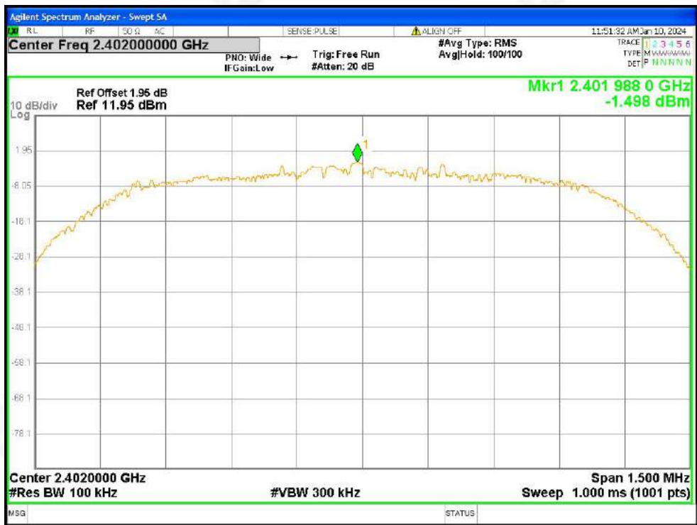
Tx. Spurious NVNT 2-DH5 2402MHz Ant1 Ref
