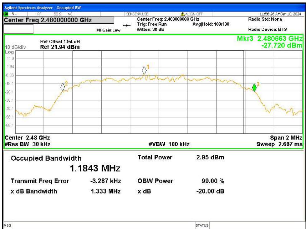
-20dB Bandwidth NVNT 2-DH5 2480MHz Ant1
