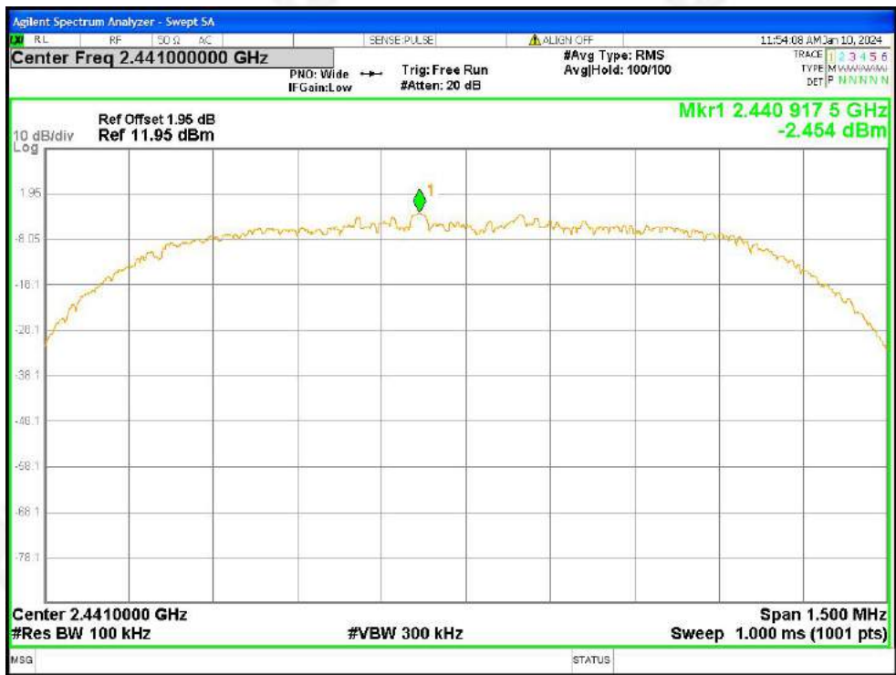
Tx. Spurious NVNT 2-DH5 2441MHz Ant1 Ref
