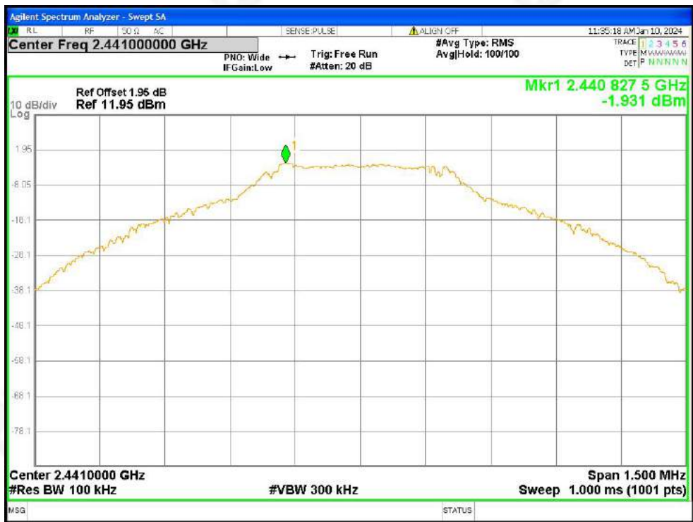
Tx. Spurious NVNT 1-DH5 2441MHz Ant1 Ref
