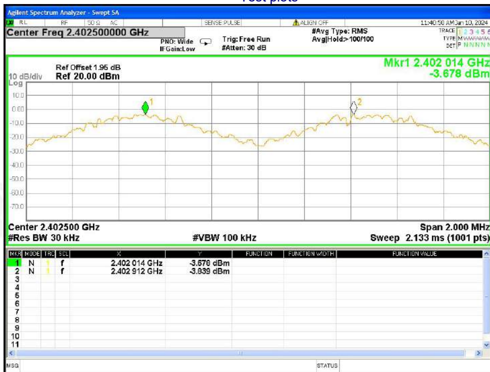
CFS NVNT 1-DH5 2402MHz Ant1
