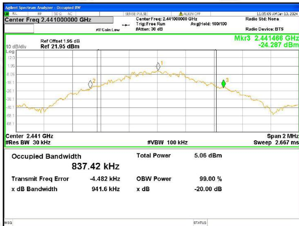
-20dB Bandwidth NVNT 1-DH5 2441MHz Ant1
