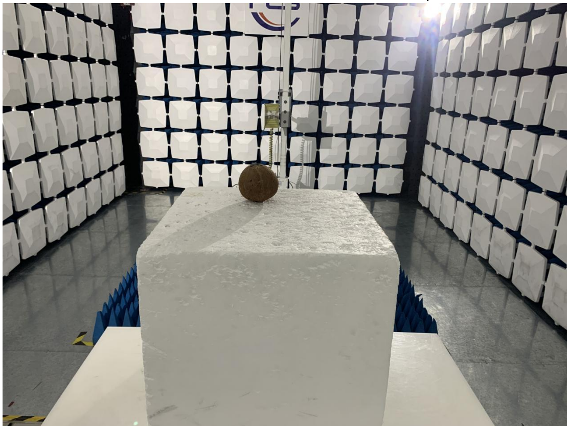
Above 1GHz for radiated emission test setup
