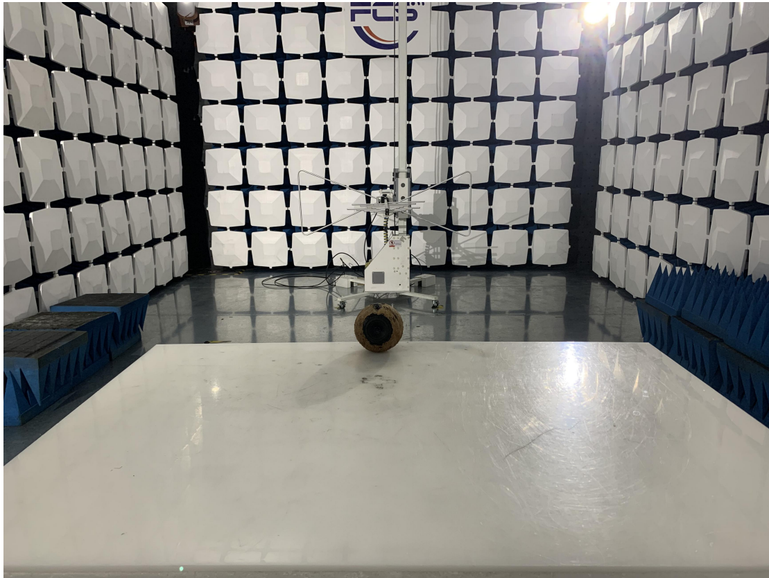
Below 1GHz for radiated emission test setup
