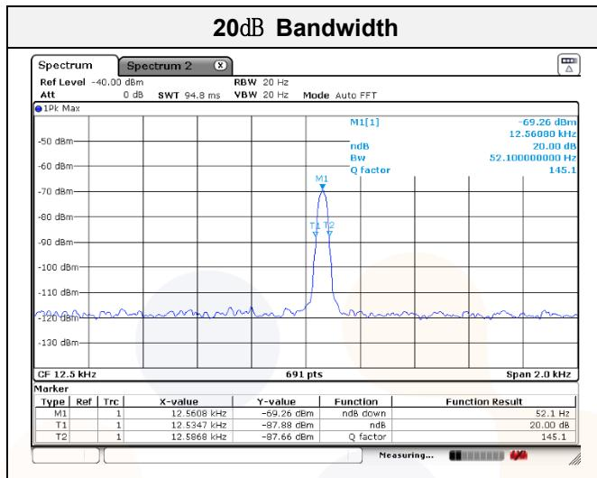
Note. Because the measured signal is CW/CW-like, adjusting the RBW per C63.10 would not be practical since measured bandwidth will always follow the RBW and the result will be approximately twice the RBW.
