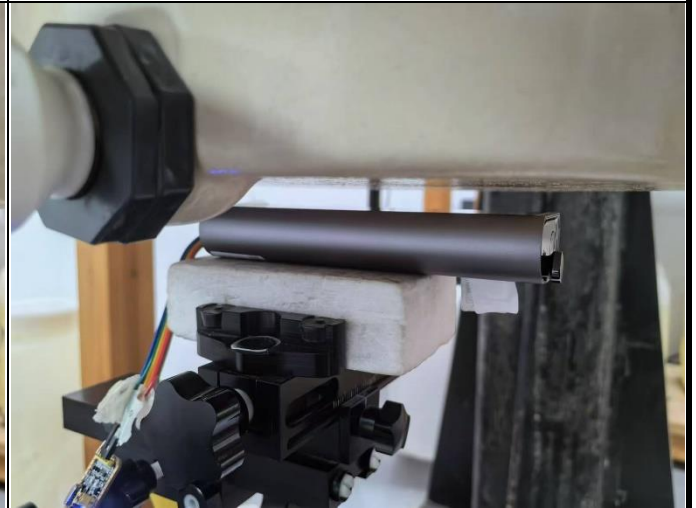
Front Face of EUT + Probe with 10 mm Gap
