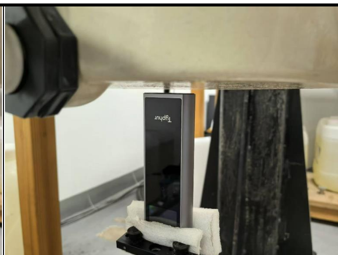
Bottom Side of EUT+ Probe with 10mm Gap
