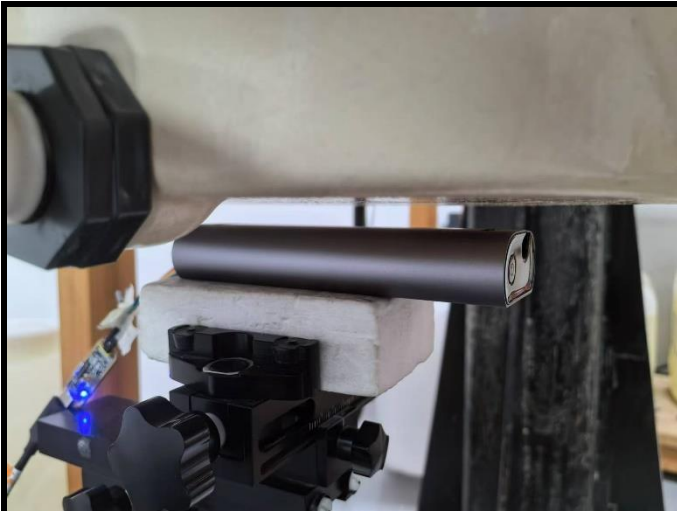
Rear Face of EUT with 10 mm Gap
