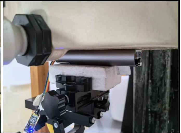
Front Face of EUT + Probe with 0 mm Gap
