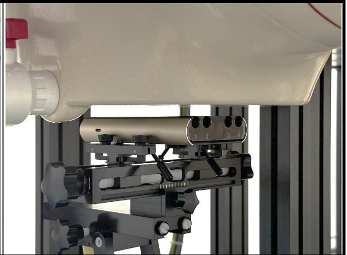
Rear Face of EUT with 10mm Gap
