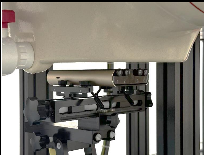
Rear Face of EUT + Probe with 10mm Gap
