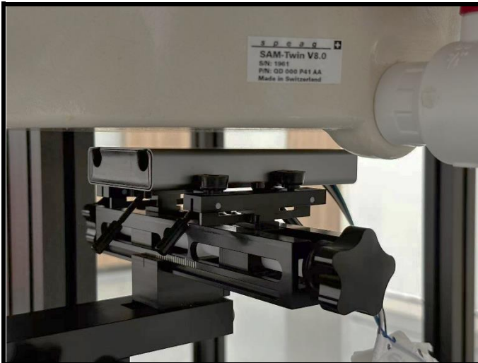
Rear Face of EUT with 10mm Gap
