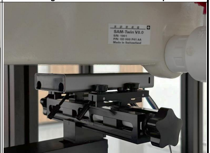
Front Face of EUT with 10mm Gap
