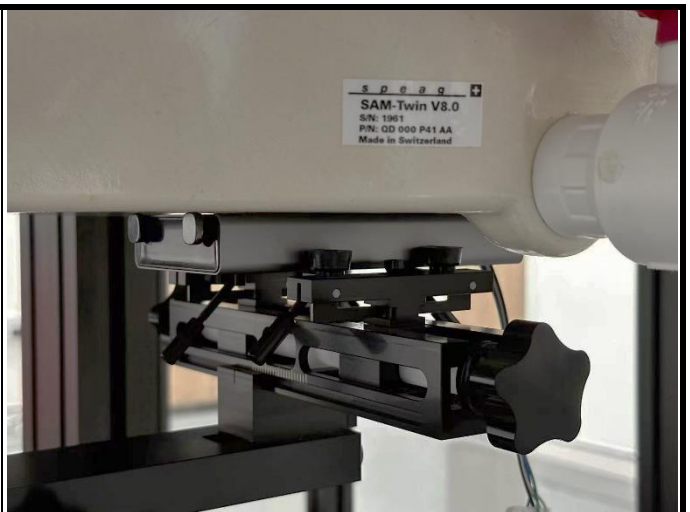
Rear Face of EUT + Probe with 0 cm Gap
