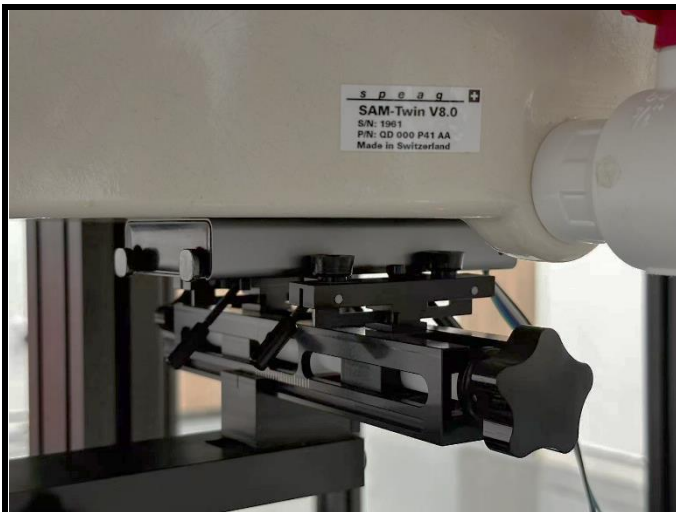
Front Face of EUT + Probe with 0 cm Gap
