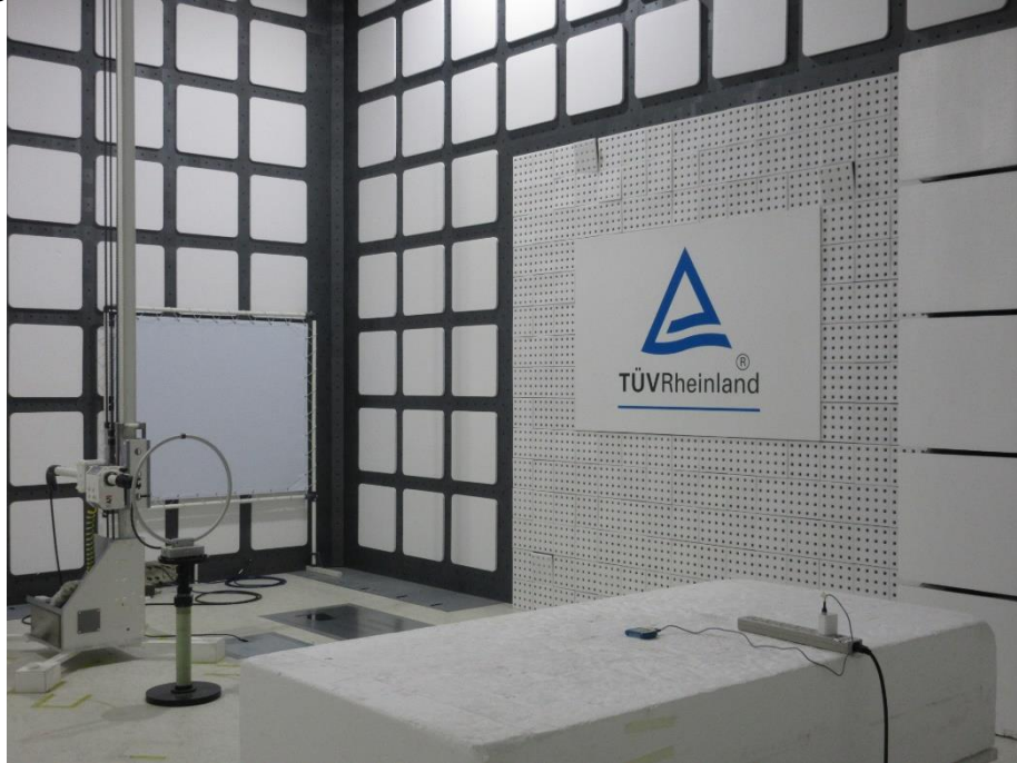
Photograph 4: Test Setup for Spurious Emissions (Back View 2)
