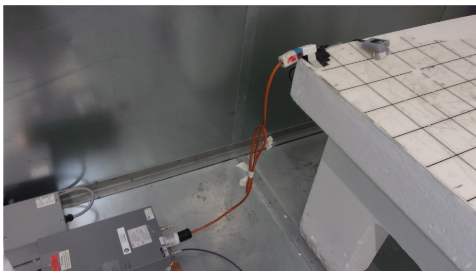
Photo 1.3-1 – Conducted AC Emissions
