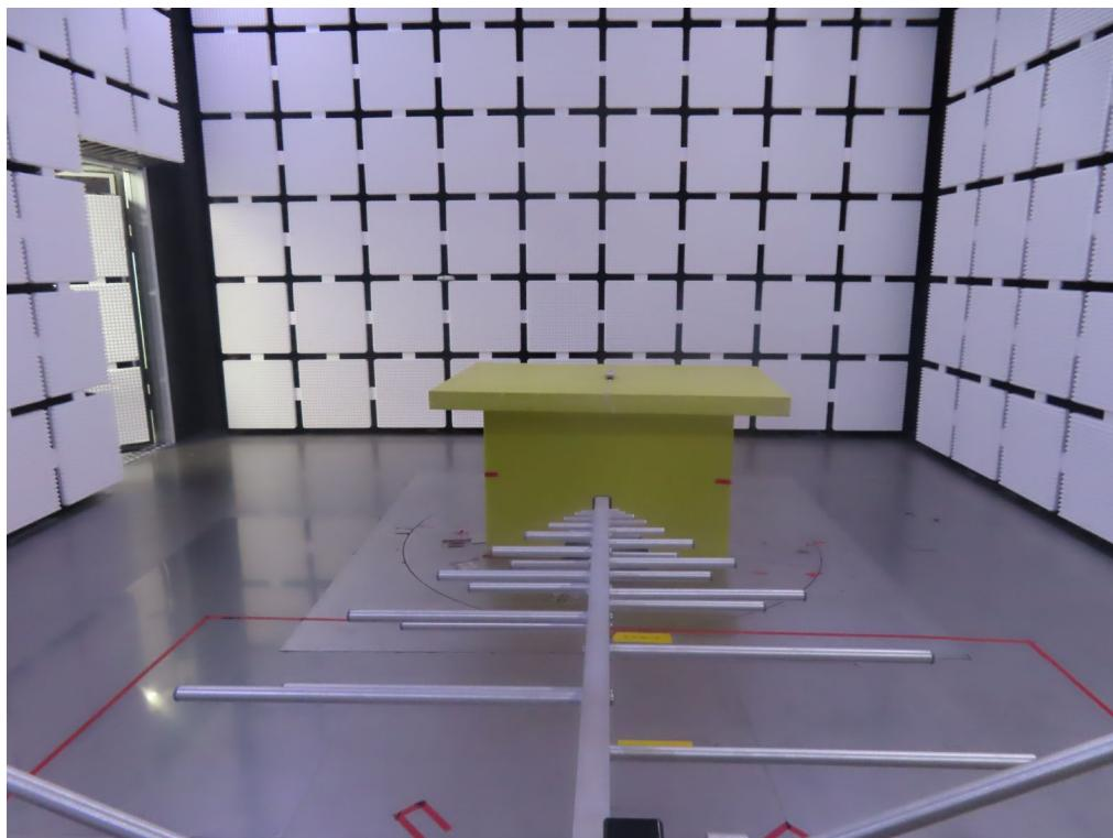
**Radiated Emissions Test Photos****Above 1 GHz**
