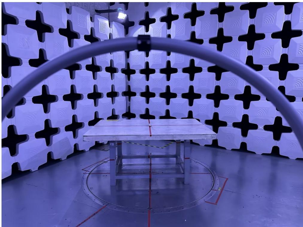
**Radiated Emissions Test Photos****30 MHz to 1 GHz**
