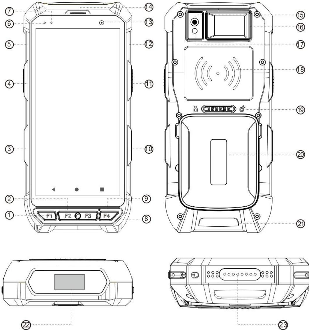
①F1 ②F2 ③Volume ④Reserved Button ⑤USB port ⑥Blue Led Indicator ⑦Red LED indicator ⑧F3 ⑨F4 ⑩Power Button ⑪Reserved Button ⑫Reserved Pogo Pin ⑬Front Camera ⑭Receiver ⑮Rear Camera ⑯Label ⑰Flashlight ⑱RFID Reading Area ⑲Battery Cover Locker ⑳Battery Cover ㉑Wrist Strap Locker ㉒Barcode Scan Window ㉓Cradle Pogo Pin Connector
