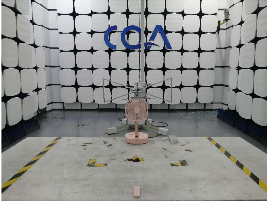
Radiated emission Test Setup (30MHz~1GHz)
