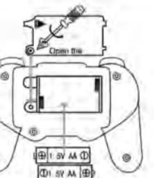
Unscrew counter clockwise to open the battery compartment cover install 2X1.5V"AA" batteries (batteries not included) into the battery compartment according to the given polarity, scary dodge to close the battery compartment
