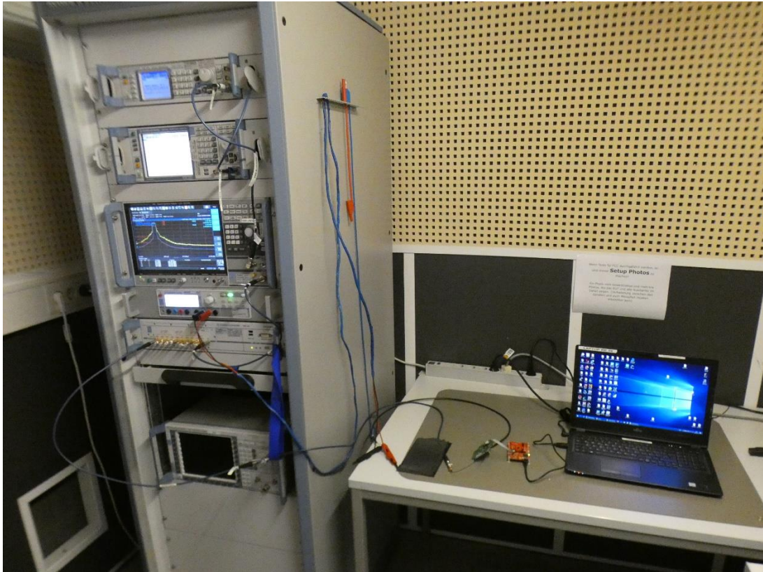
Photo 5: Test setup for conducted measurements
