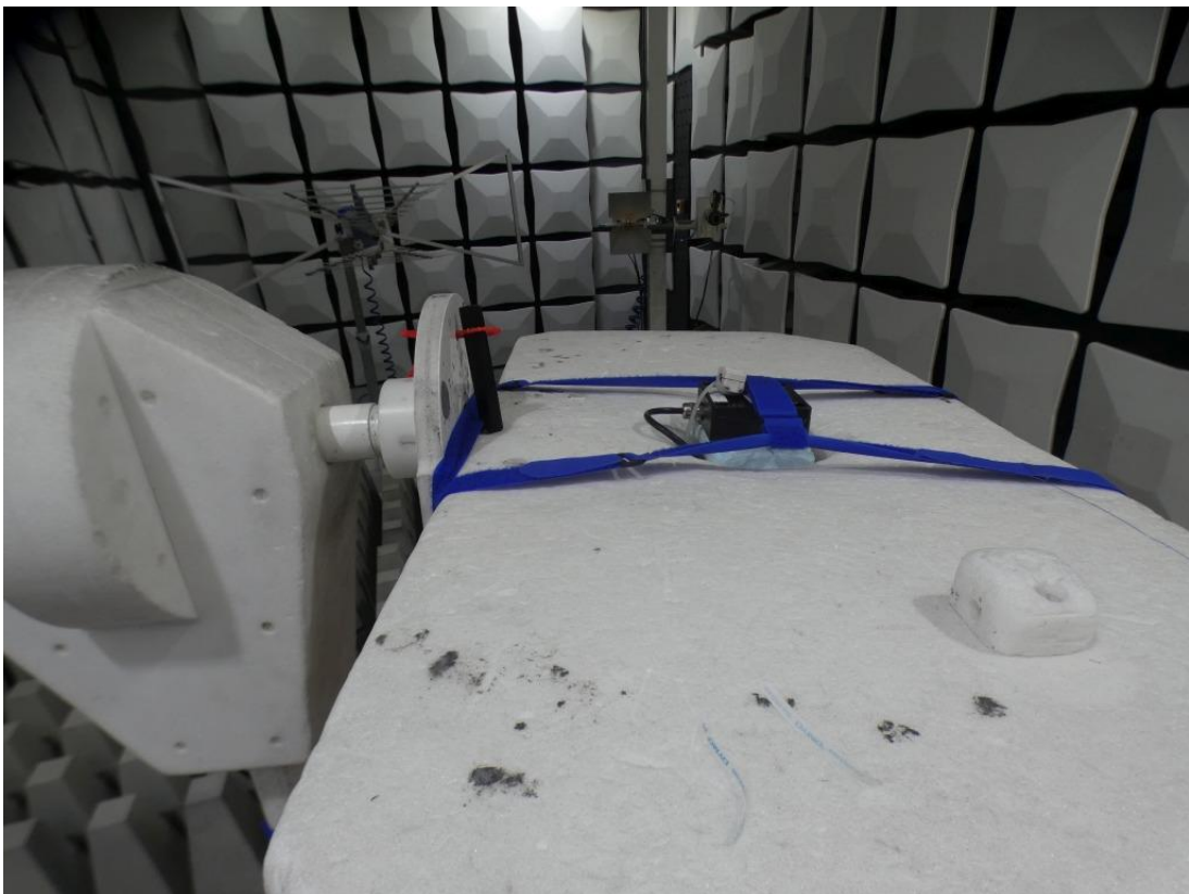
Photo 4: Test setup for radiated measurements, Band Edge Compliance
