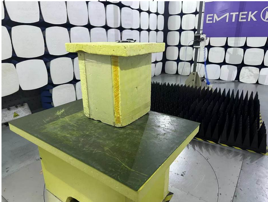
Spurious Emission Test Setup (Above 1GHz)
