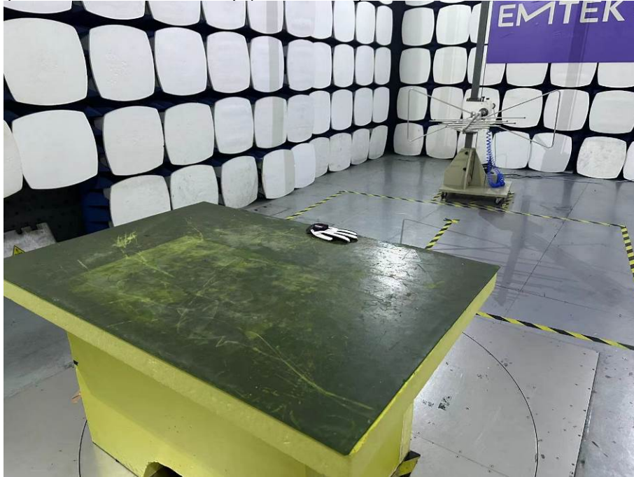
Spurious Emission Test Setup (Below 1GHz)
