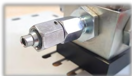
Place the second cutting ring and sealable nut opposite side - thread to the left side of plate
