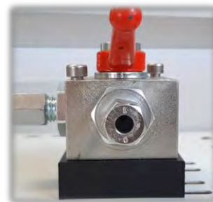
Holding the small plate using the hand tighten preliminary the three way valve, putting a spacer under it. Tighten it just to keep together all the parts allowing for horizontal movement of the valve.
