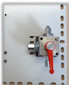
Remember to place the valve with one port to be directed to the left side of the plate.
