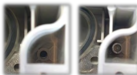
Align device onto plate to fit with the mounting holes with rivet nuts. Use the attached screws M5x12 to attach the device to plate.
