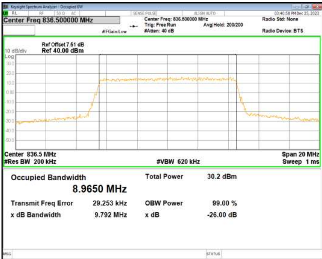
Band5 QPSK BW=10MHz Channel=20600 RB Size=50 Position=#0
