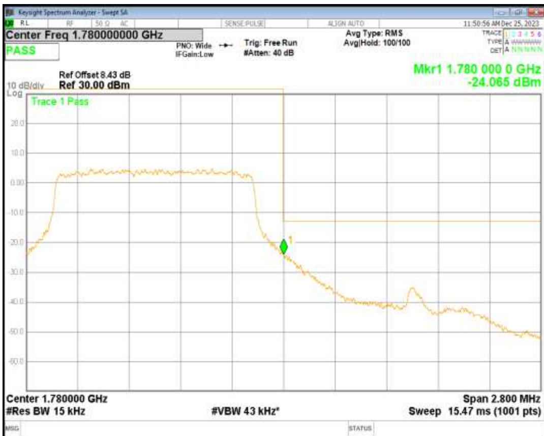
Band66 16QAM BW=3MHz Channel=131987 RB Size=15 Position=#0
