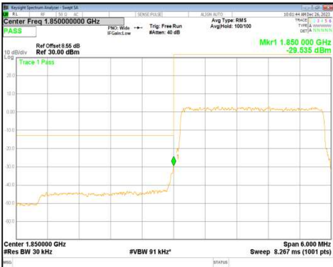
Band2 QPSK BW=3MHz Channel=19185 RB Size=15 Position=#0
