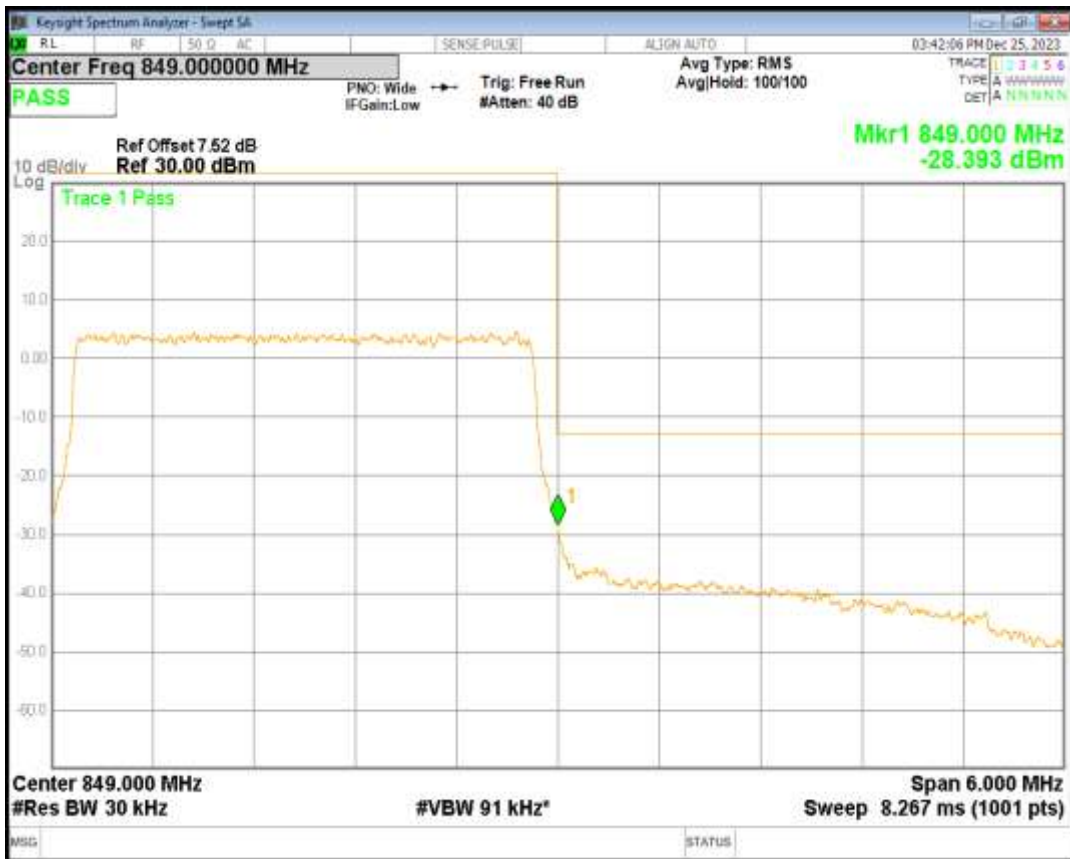
Band5 16QAM BW=3MHz Channel=20635 RB Size=15 Position=#0
