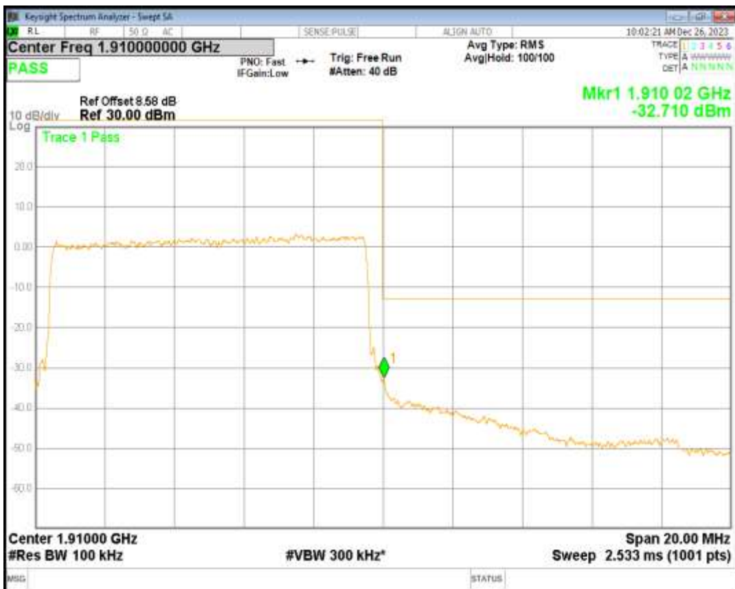
Band2 QPSK BW=15MHz Channel=18675 RB Size=75 Position=#0
