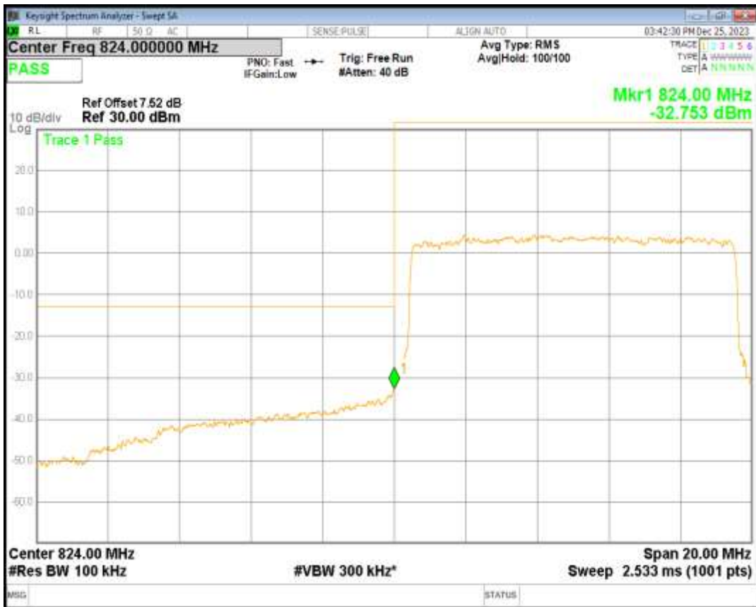
Band5 QPSK BW=10MHz Channel=20600 RB Size=50 Position=#0
