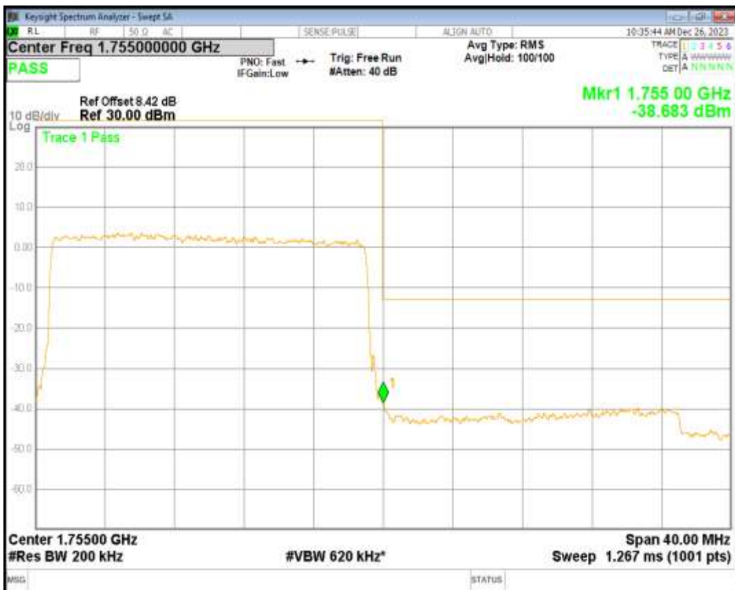
Band5 QPSK BW=1.4MHz Channel=20407 RB Size=6 Position=#0
