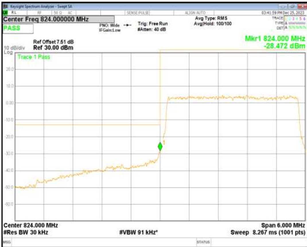
Band5 16QAM BW=3MHz Channel=20415 RB Size=15 Position=#0
