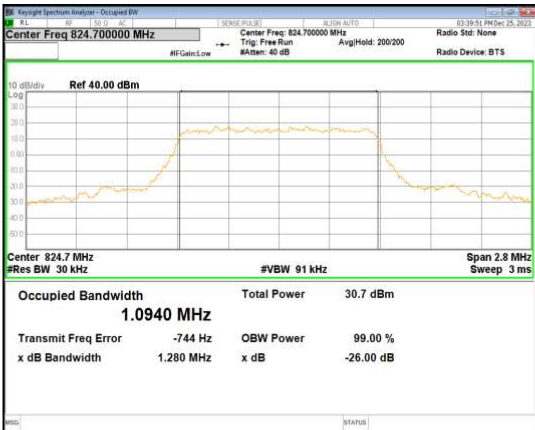
Band5 16QAM BW=1.4MHz Channel=20407 RB Size=6 Position=#0
