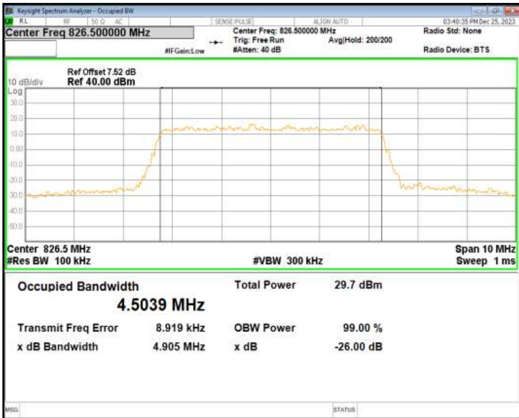
Band5 QPSK BW=5MHz Channel=20525 RB Size=25 Position=#0
