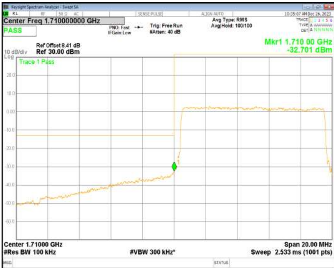
Band4 QPSK BW=10MHz Channel=20350 RB Size=50 Position=#0
