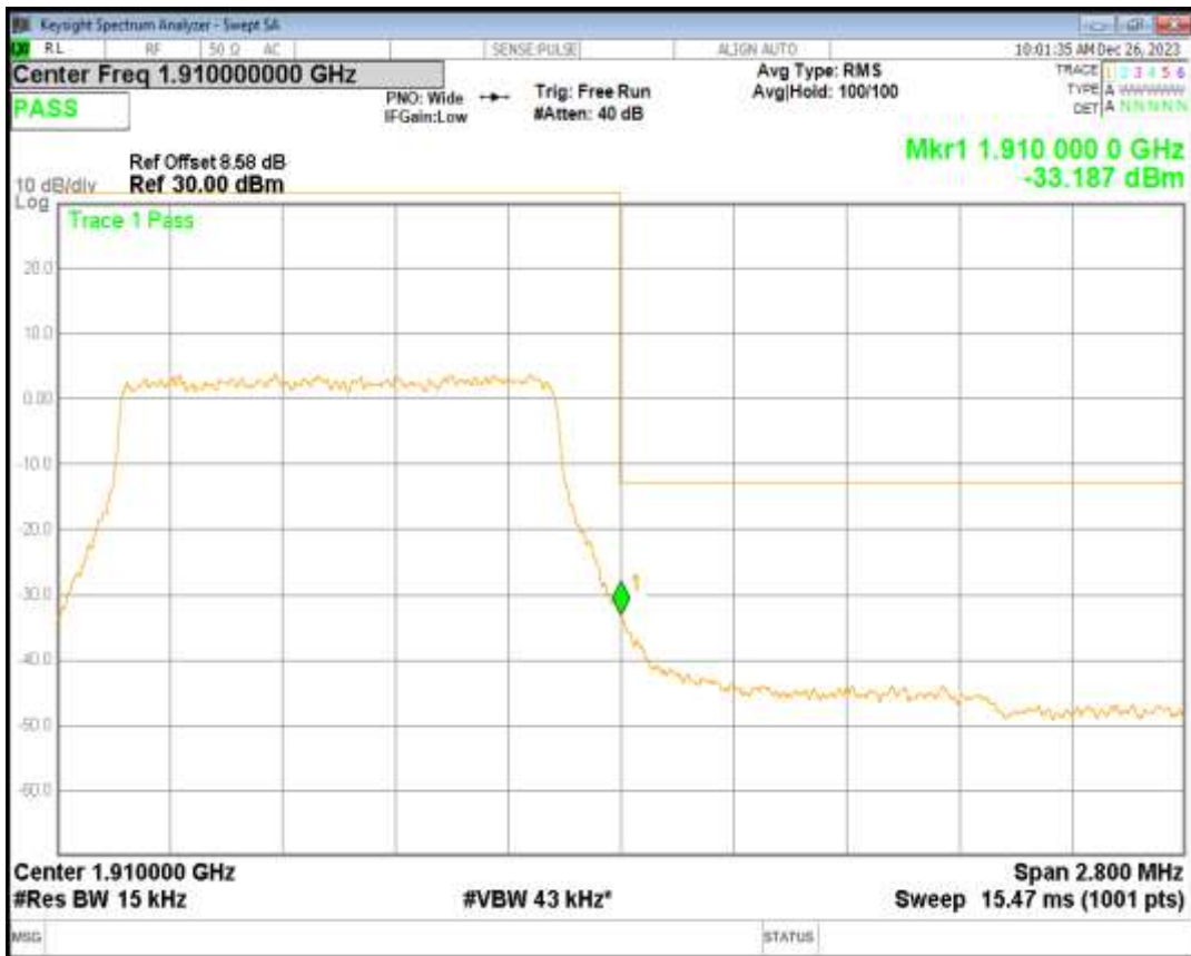
Band2 16QAM BW=1.4MHz Channel=19193 RB Size=6 Position=#0
