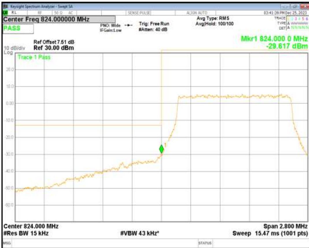
Band5 16QAM BW=1.4MHz Channel=20407 RB Size=6 Position=#0
