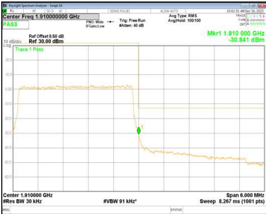
Band2 16QAM BW=3MHz Channel=19185 RB Size=15 Position=#0
