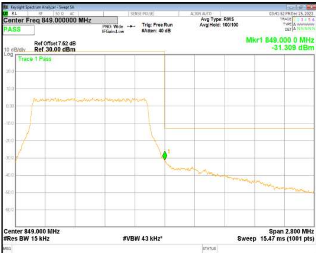
Band5 QPSK BW=3MHz Channel=20415 RB Size=15 Position=#0
