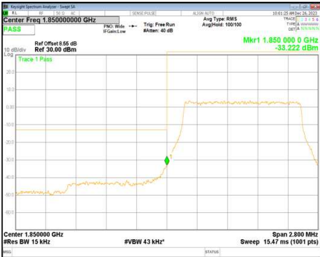
Band2 16QAM BW=1.4MHz Channel=18607 RB Size=6 Position=#0
