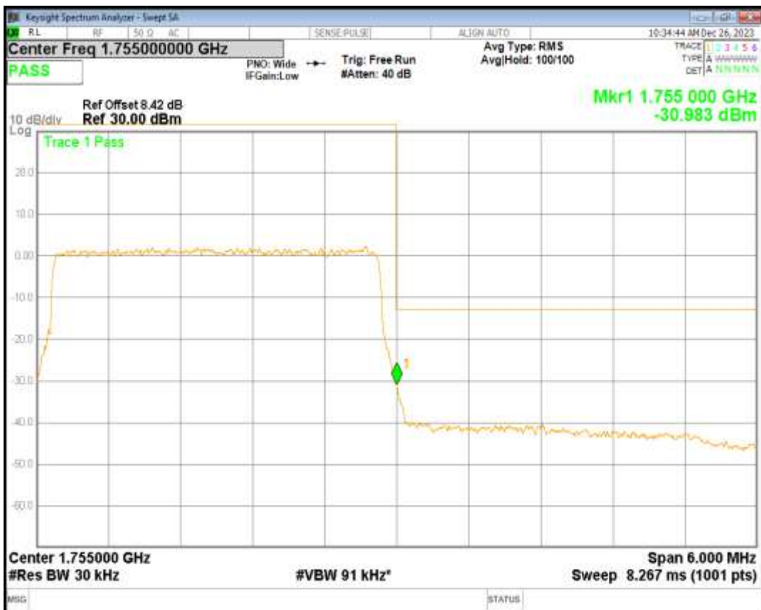
Band4 QPSK BW=5MHz Channel=19975 RB Size=25 Position=#0
