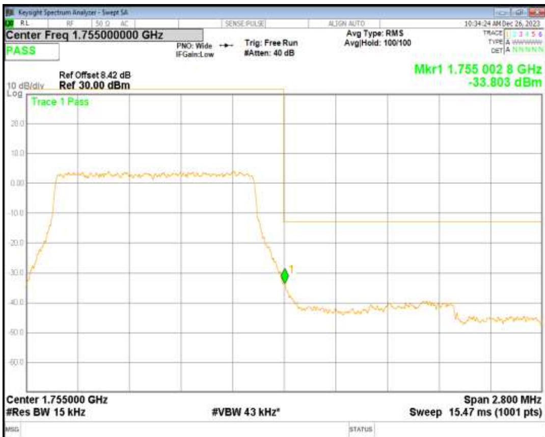
Band4 QPSK BW=3MHz Channel=19965 RB Size=15 Position=#0
