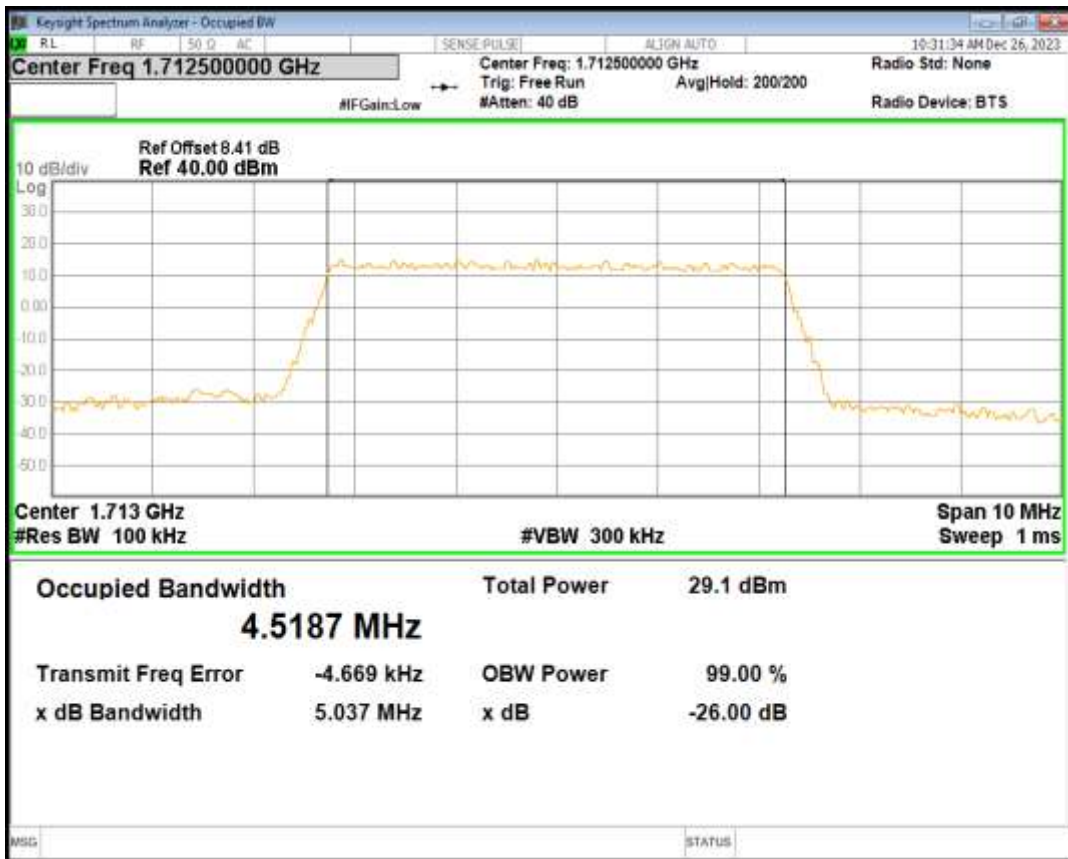
Band4 16QAM BW=5MHz Channel=19975 RB Size=25 Position=#0
