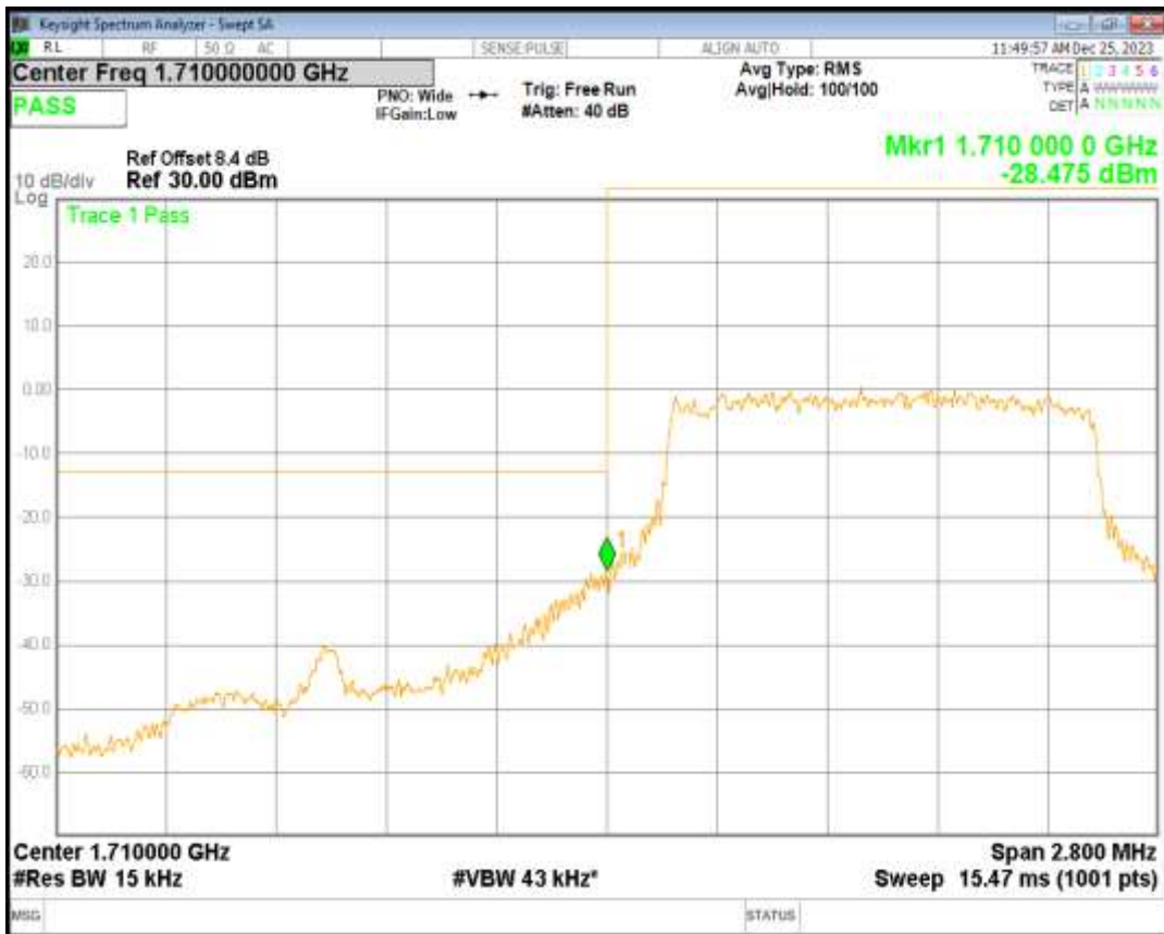
Band66 16QAM BW=1.4MHz Channel=132665 RB Size=6 Position=#0
