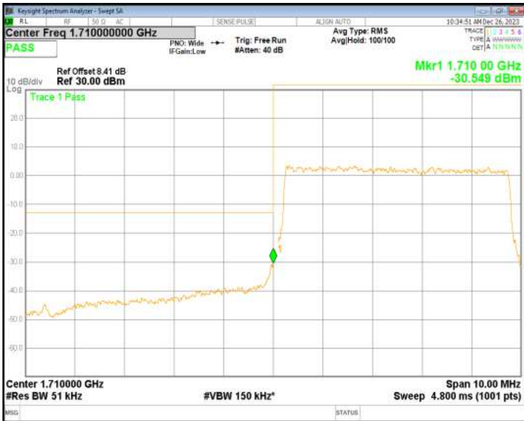
Band4 16QAM BW=5MHz Channel=19975 RB Size=25 Position=#0
