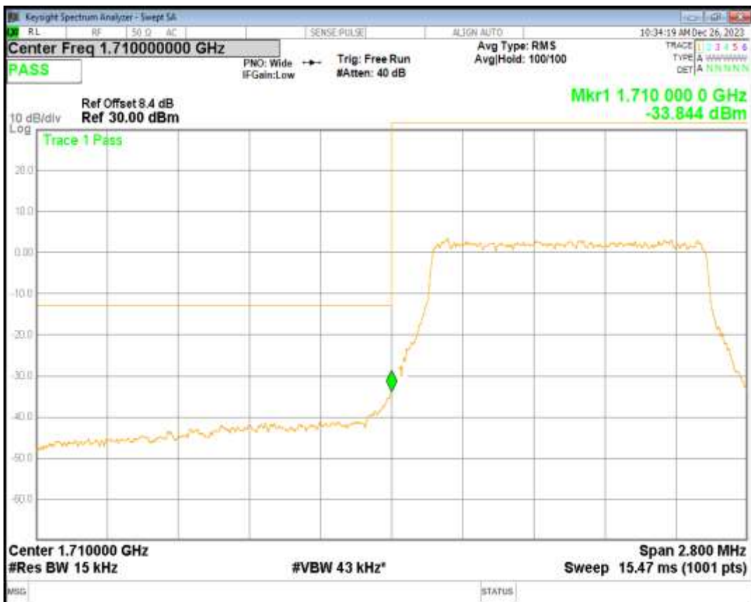
Band4 16QAM BW=1.4MHz Channel=20393 RB Size=6 Position=#0
