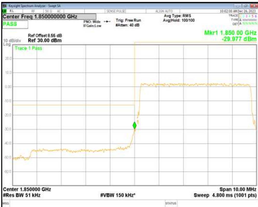
Band2 QPSK BW=5MHz Channel=19175 RB Size=25 Position=#0
