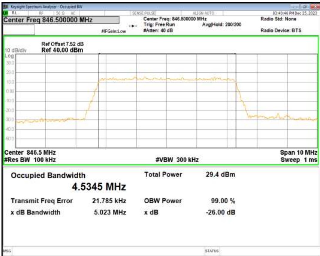
Band5 QPSK BW=10MHz Channel=20450 RB Size=50 Position=#0
