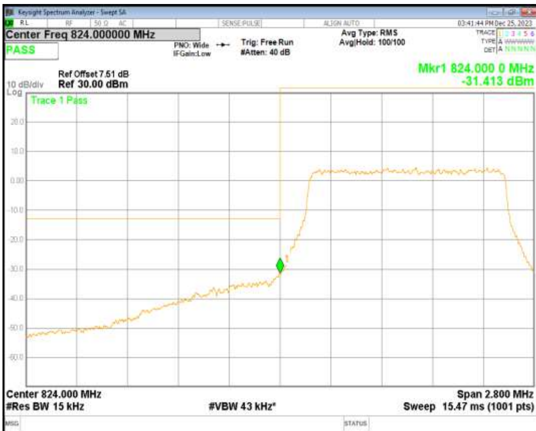
Band5 QPSK BW=1.4MHz Channel=20643 RB Size=6 Position=#0
