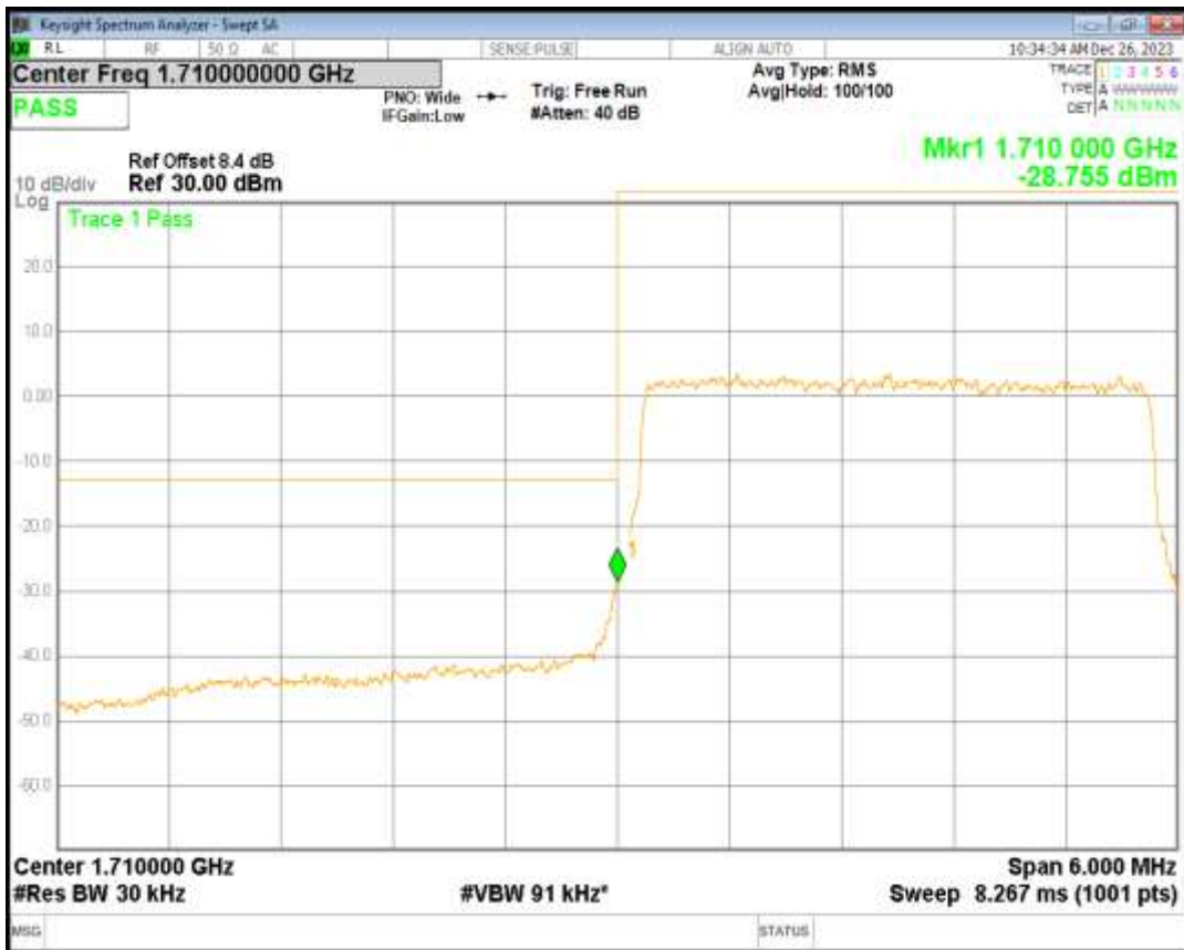
Band4 16QAM BW=3MHz Channel=19965 RB Size=15 Position=#0
