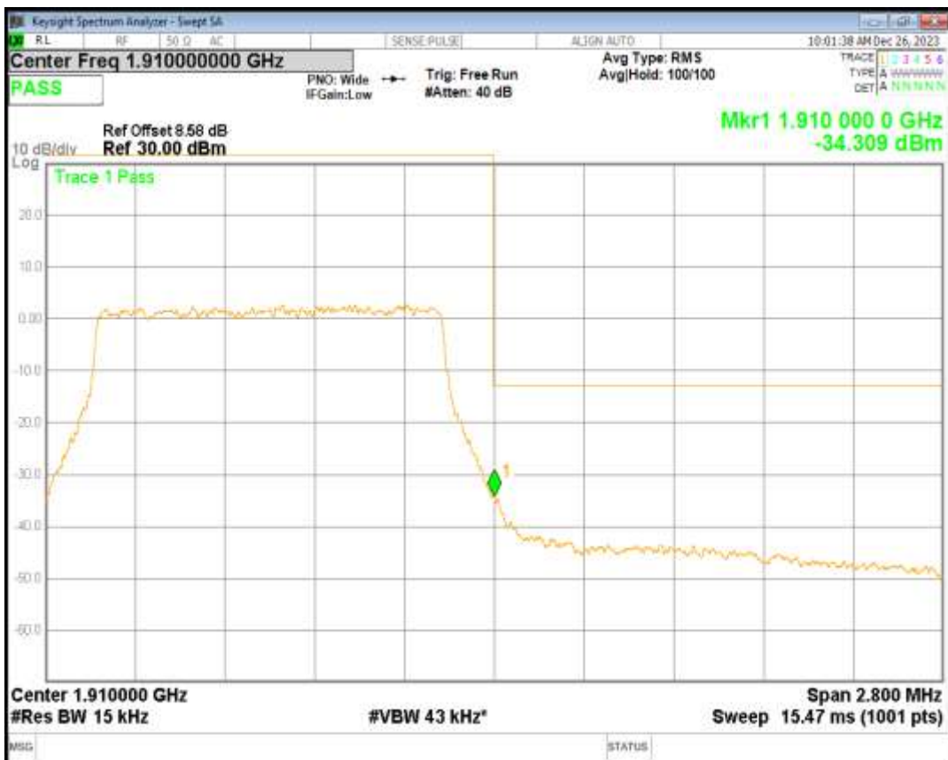
Band2 16QAM BW=3MHz Channel=18615 RB Size=15 Position=#0
