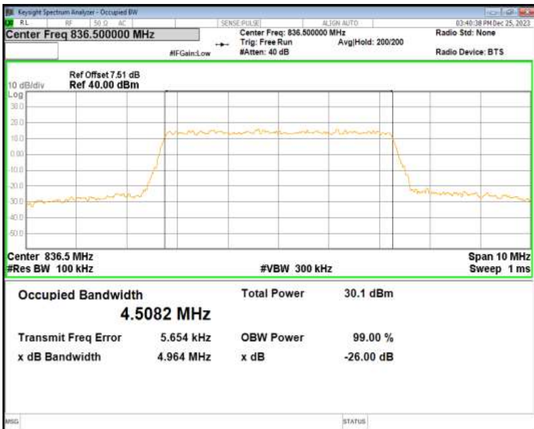
Band5 16QAM BW=5MHz Channel=20525 RB Size=25 Position=#0
