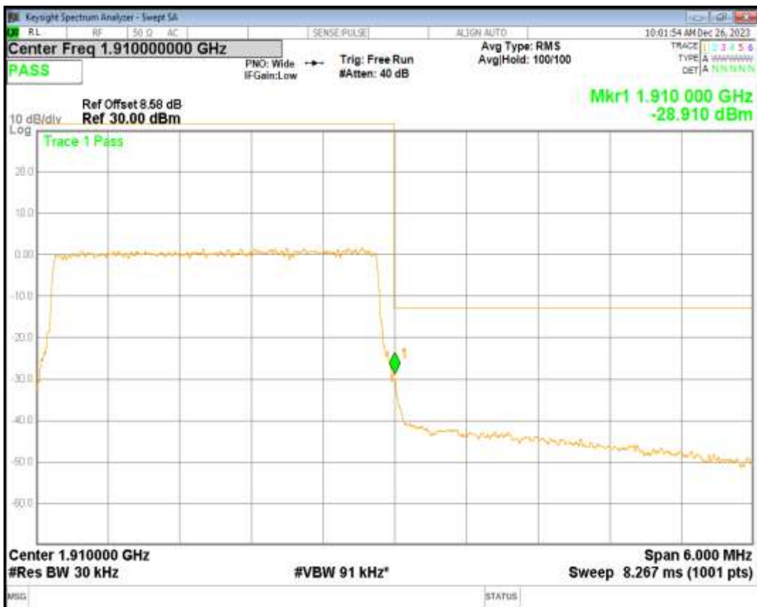
Band2 16QAM BW=5MHz Channel=18625 RB Size=25 Position=#0
