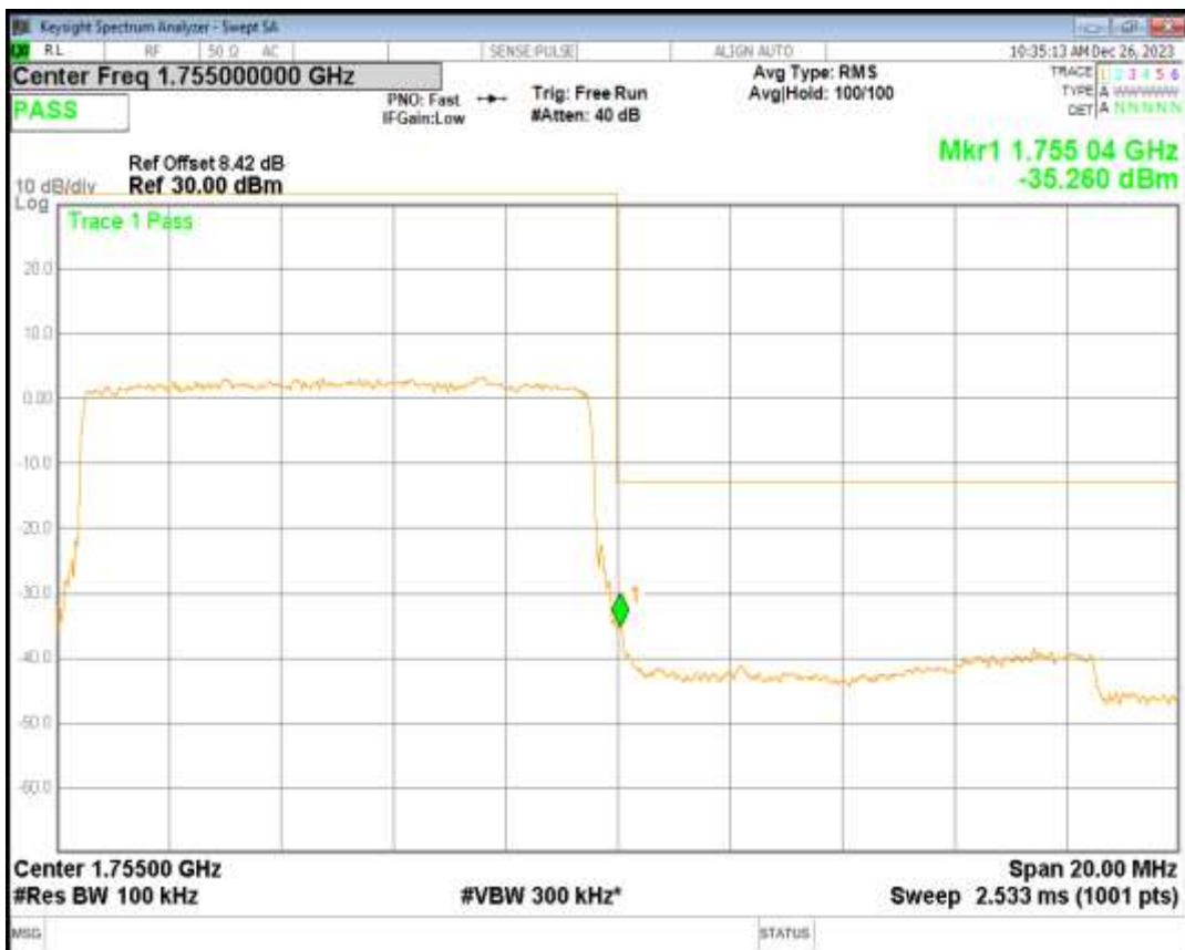
Band4 QPSK BW=15MHz Channel=20025 RB Size=75 Position=#0
