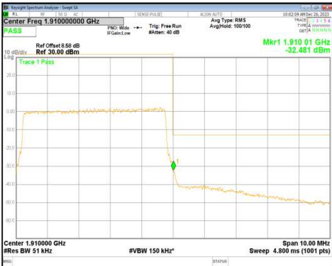
Band2 QPSK BW=10MHz Channel=18650 RB Size=50 Position=#0
