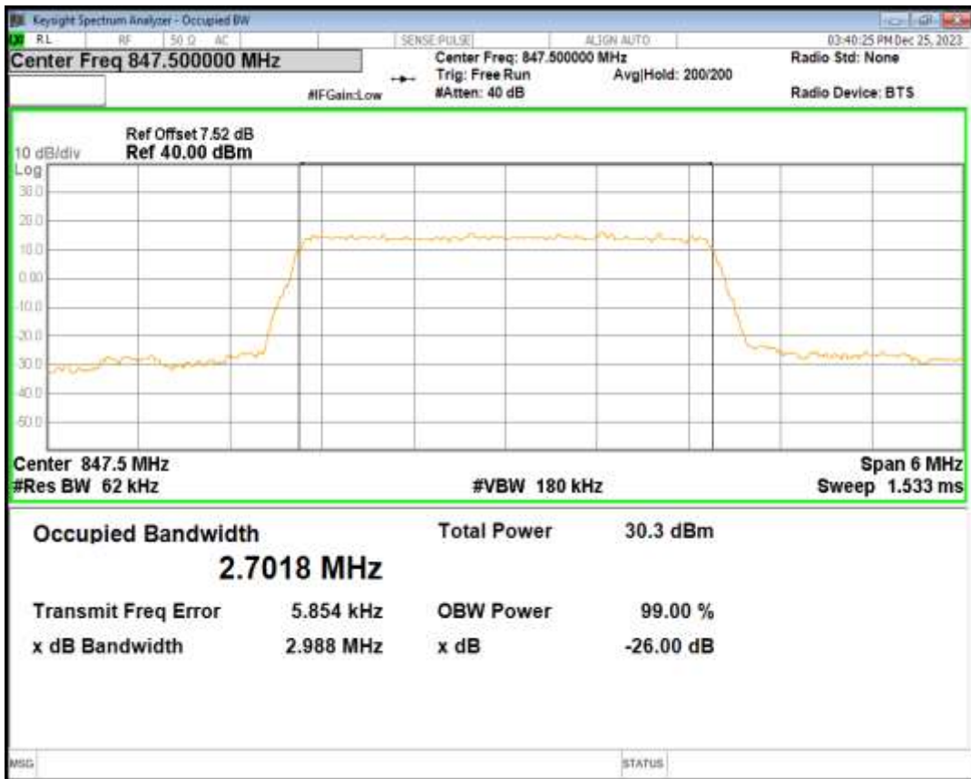
Band5 QPSK BW=5MHz Channel=20425 RB Size=25 Position=#0
