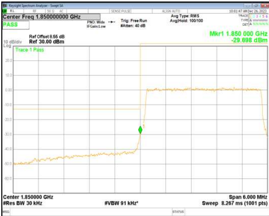
Band2 QPSK BW=3MHz Channel=18615 RB Size=15 Position=#0
