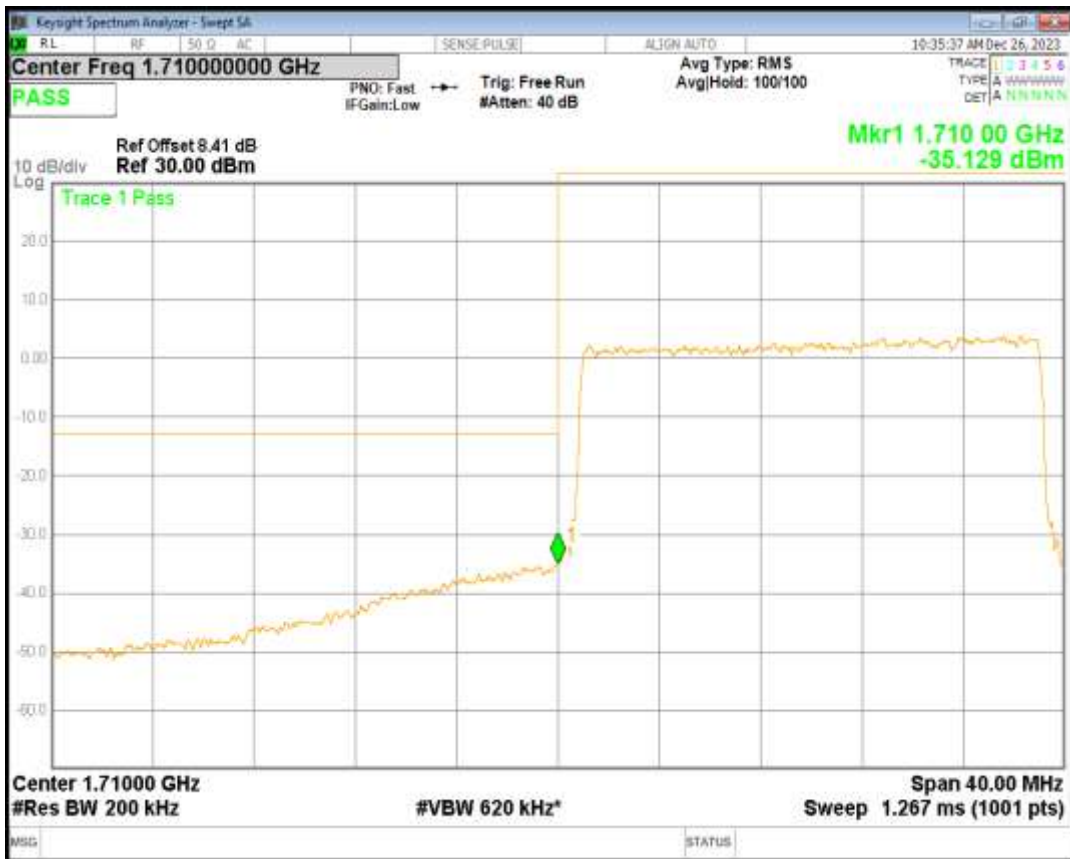
Band4 QPSK BW=20MHz Channel=20300 RB Size=100 Position=#0
