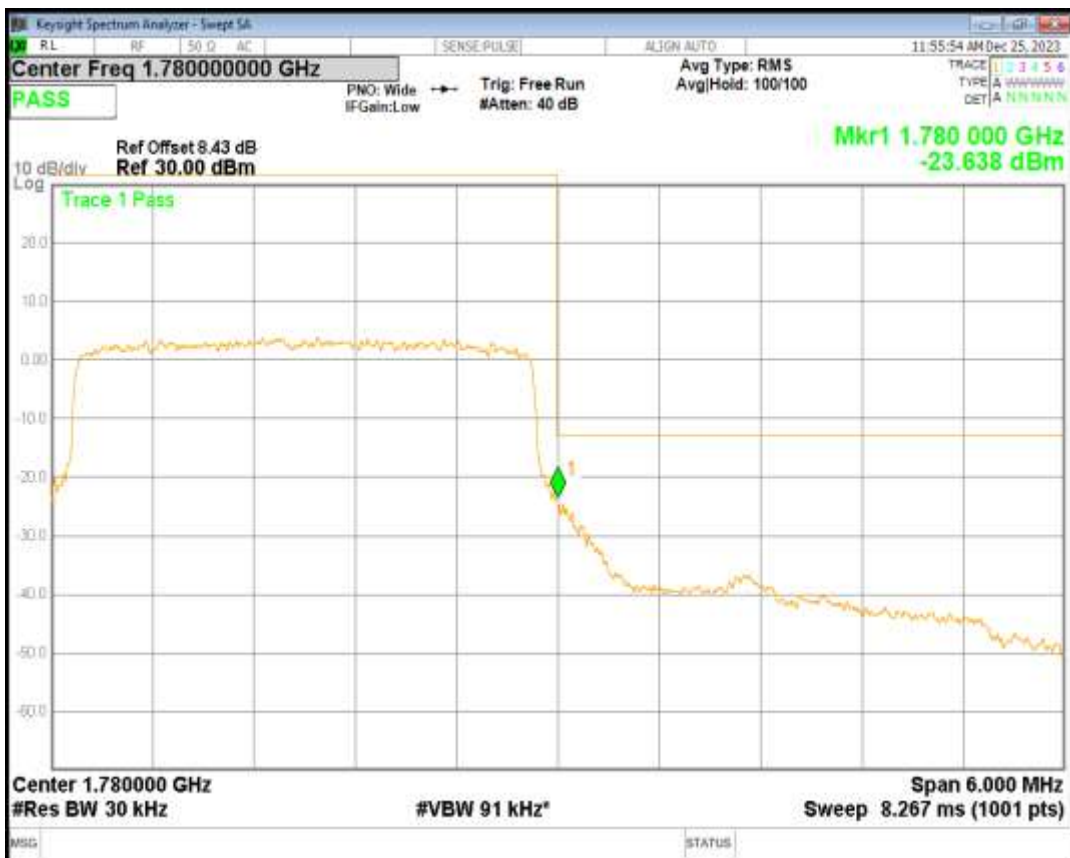
Band66 16QAM BW=5MHz Channel=131997 RB Size=25 Position=#0
