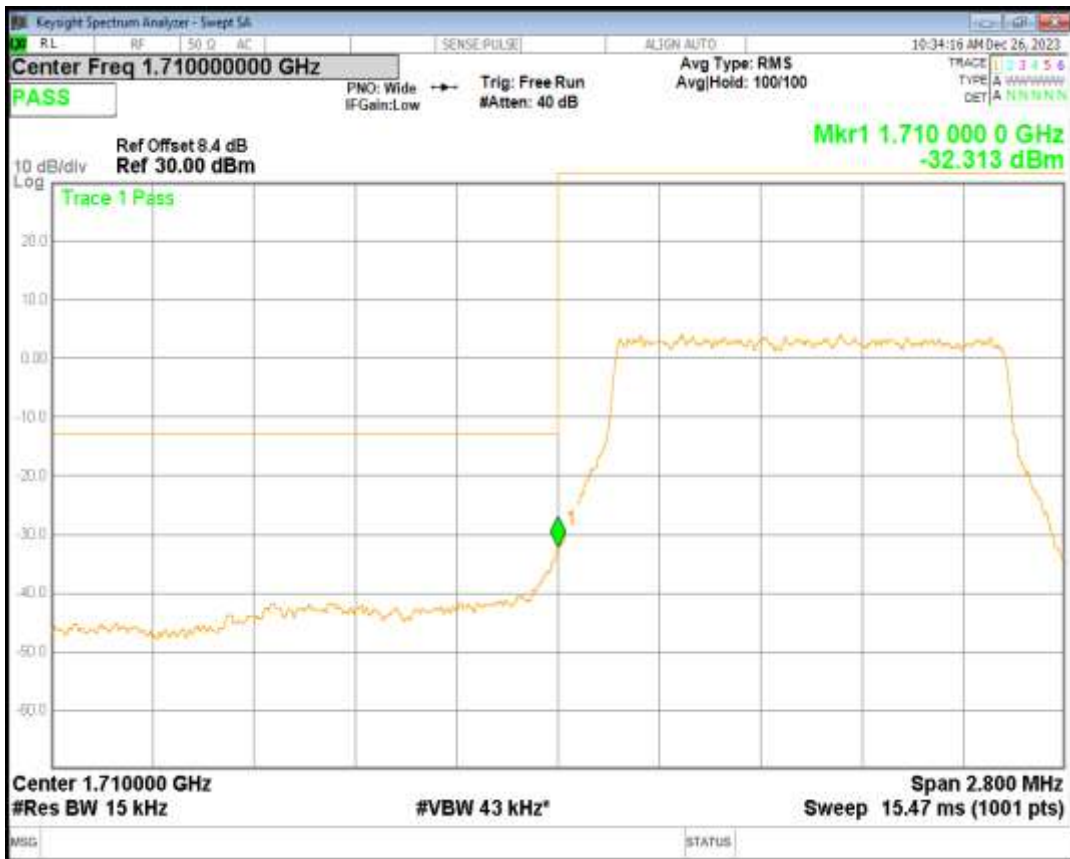
Band4 16QAM BW=1.4MHz Channel=19957 RB Size=6 Position=#0
