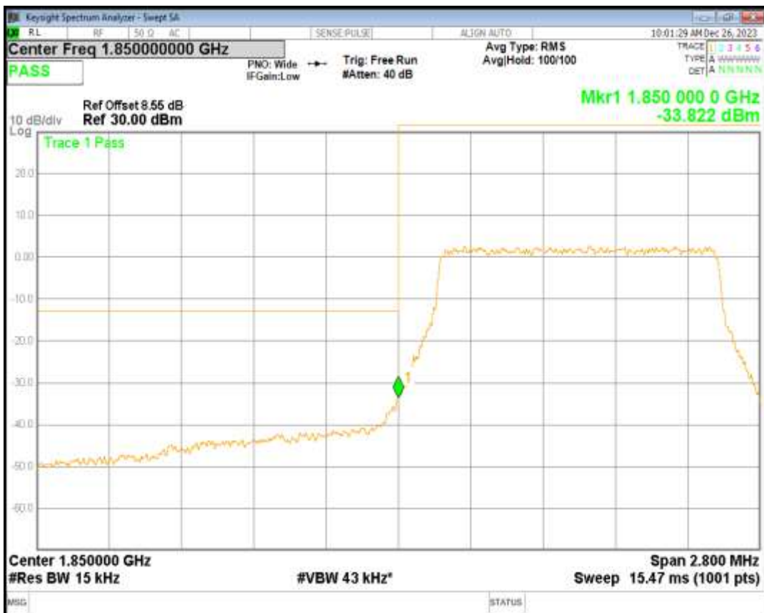
Band2 QPSK BW=1.4MHz Channel=19193 RB Size=6 Position=#0
