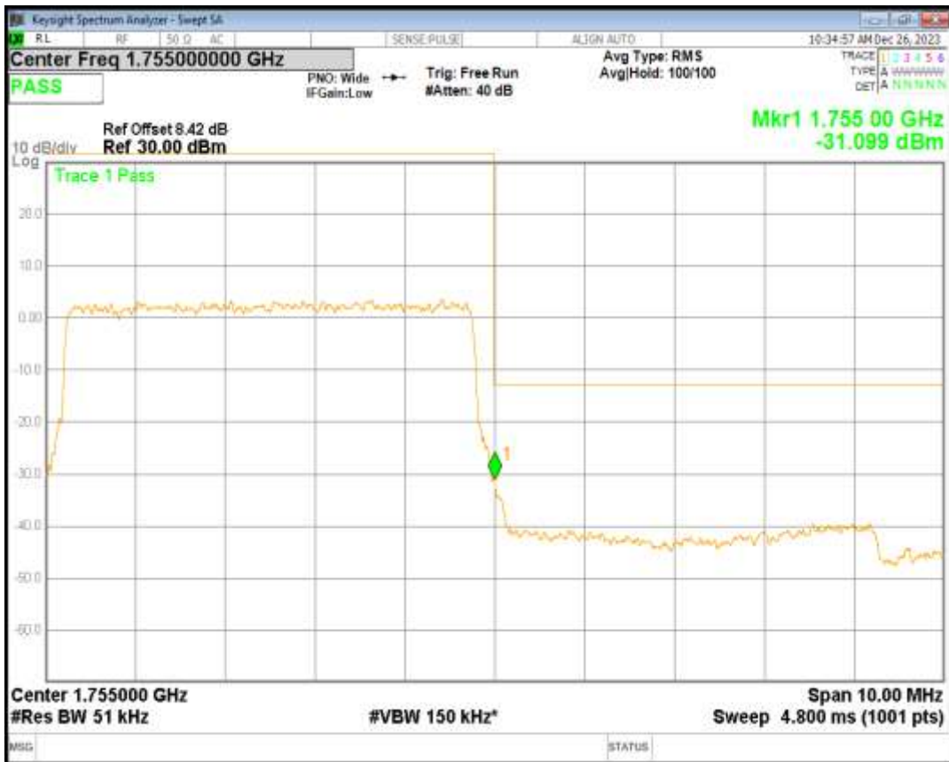
Band4 16QAM BW=5MHz Channel=20375 RB Size=25 Position=#0
