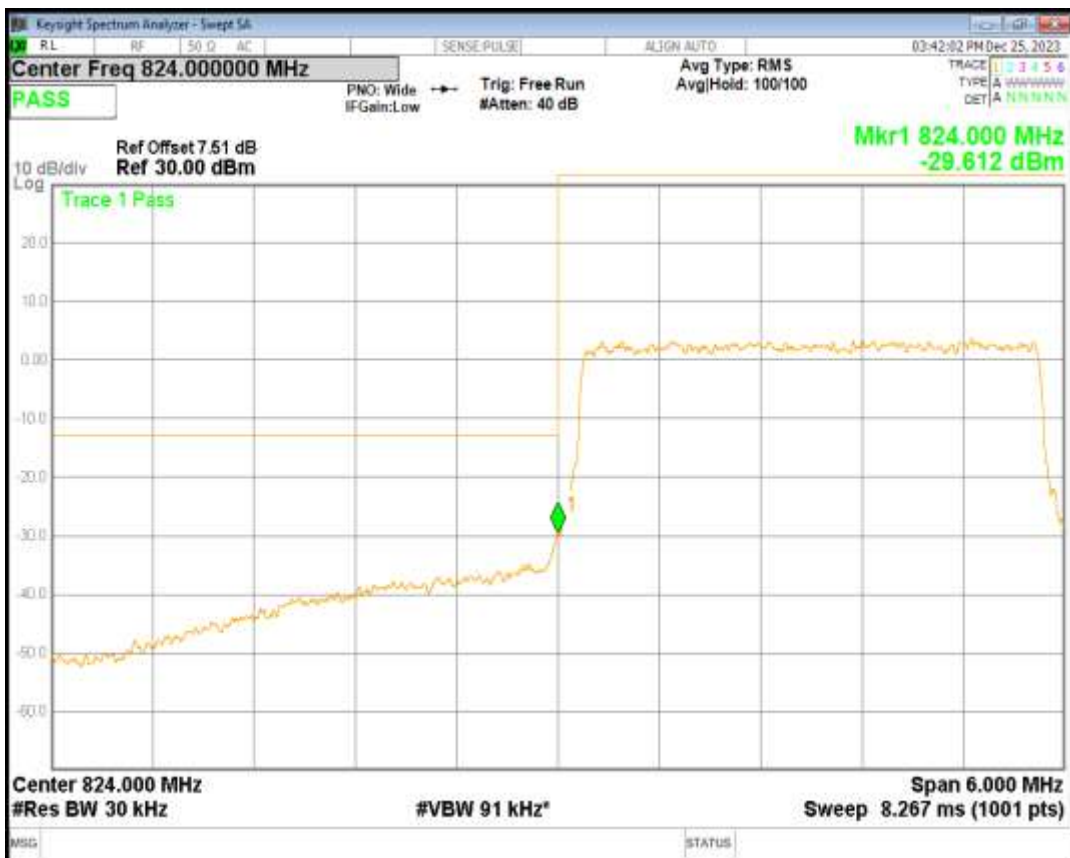
Band5 QPSK BW=3MHz Channel=20635 RB Size=15 Position=#0
