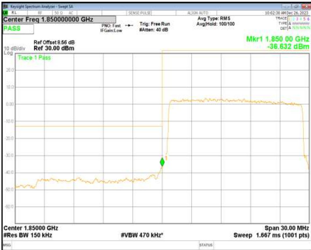
Band2 QPSK BW=15MHz Channel=19125 RB Size=75 Position=#0
