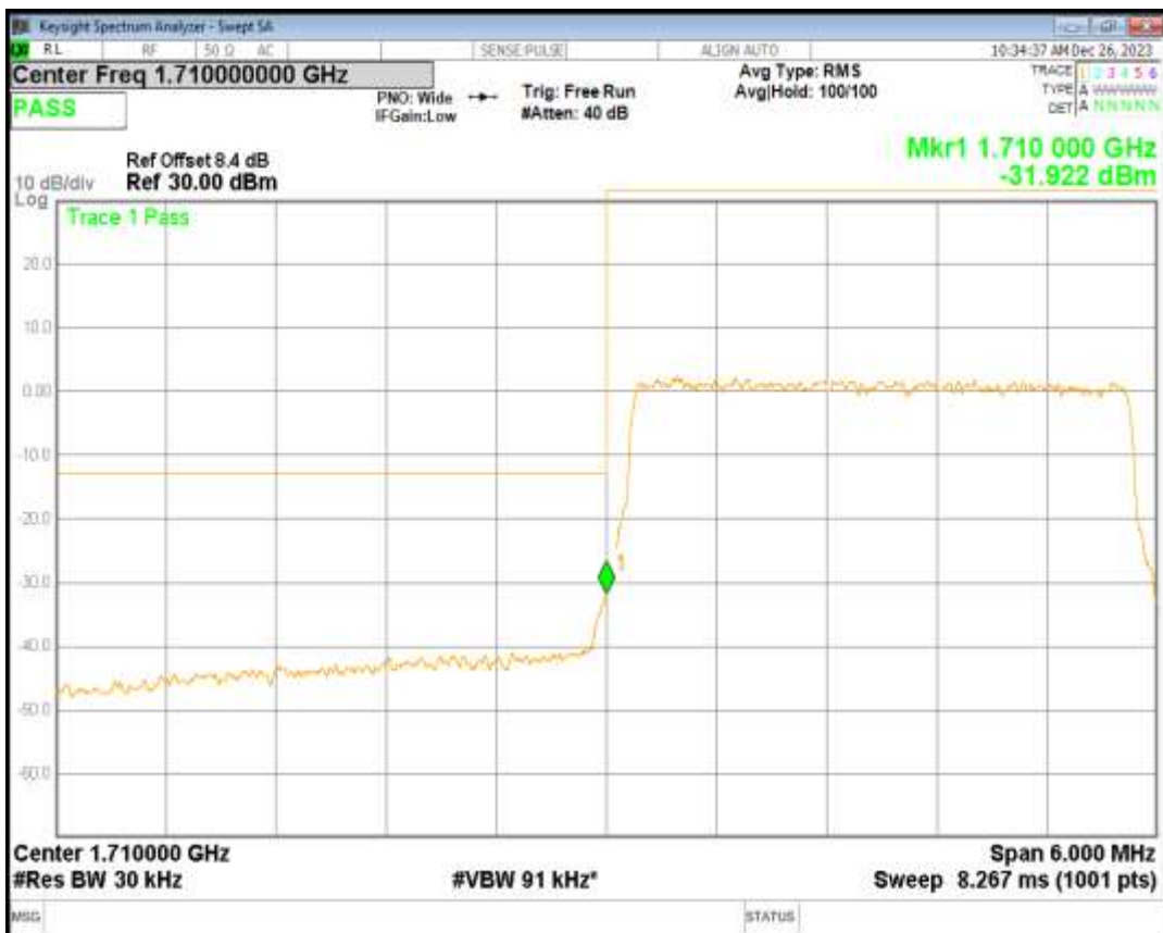
Band4 QPSK BW=3MHz Channel=20385 RB Size=15 Position=#0
