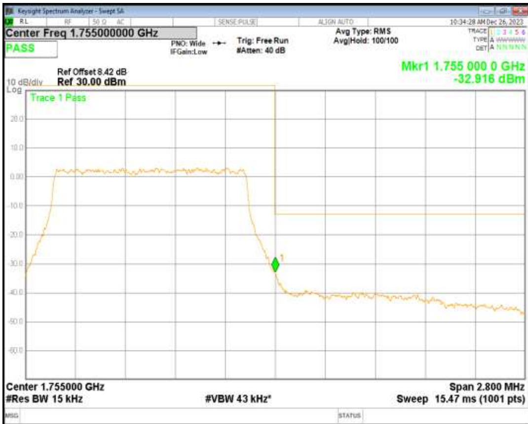
Band4 QPSK BW=1.4MHz Channel=20393 RB Size=6 Position=#0
