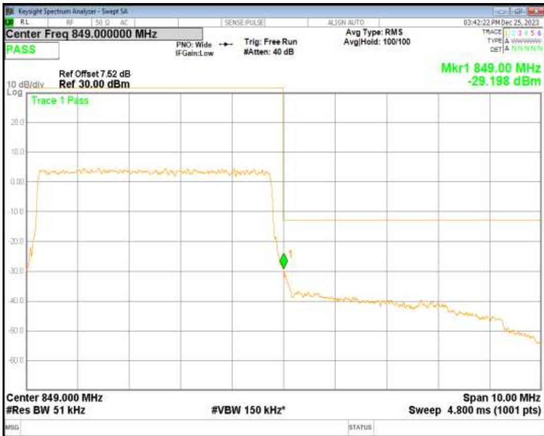
Band5 16QAM BW=5MHz Channel=20625 RB Size=25 Position=#0
