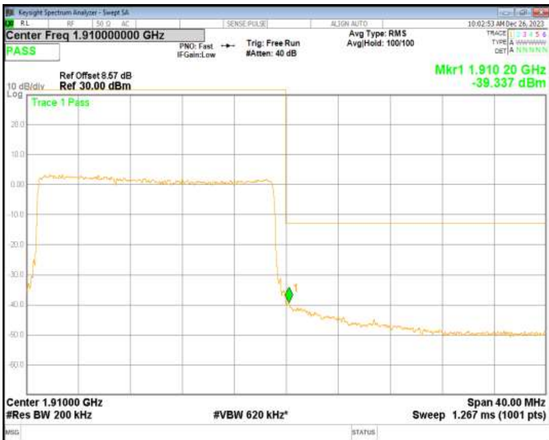
Band4 QPSK BW=1.4MHz Channel=19957 RB Size=6 Position=#0
