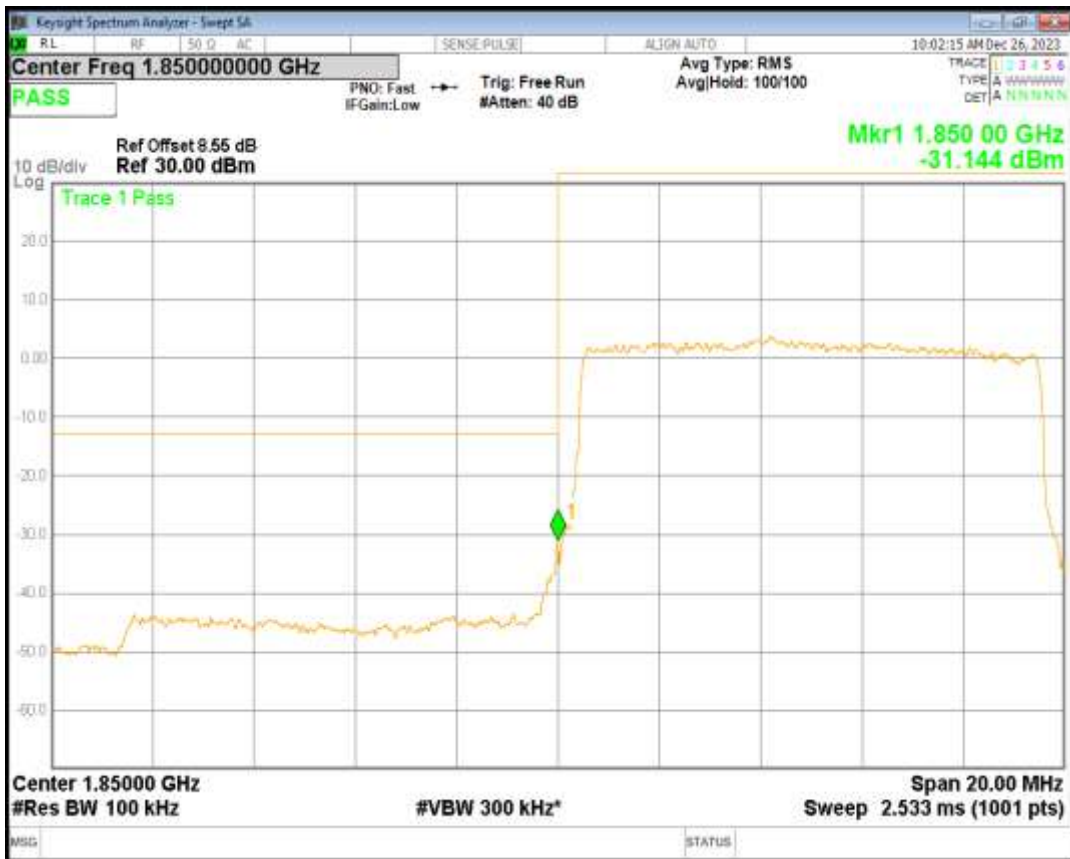
Band2 QPSK BW=10MHz Channel=19150 RB Size=50 Position=#0
