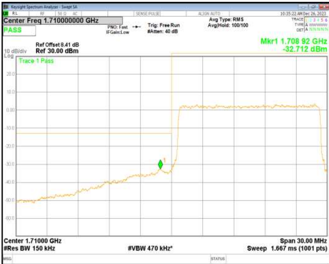
Band4 QPSK BW=15MHz Channel=20325 RB Size=75 Position=#0
