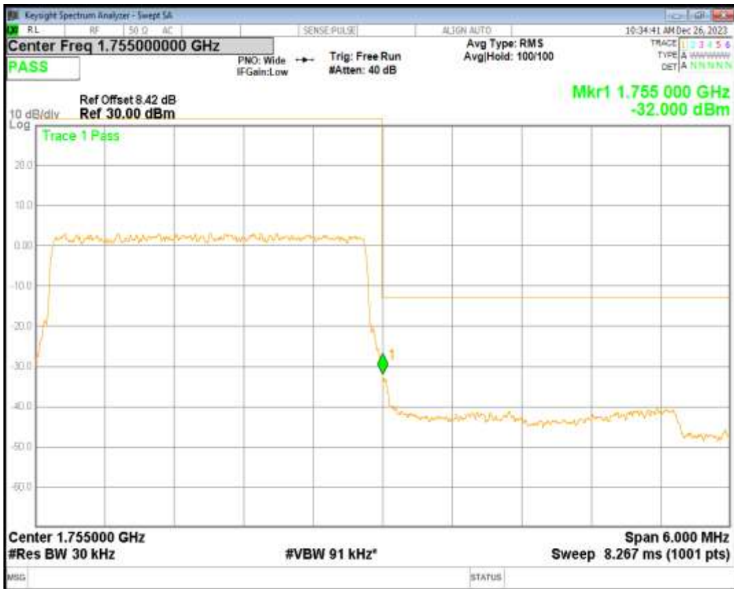
Band4 16QAM BW=3MHz Channel=20385 RB Size=15 Position=#0
