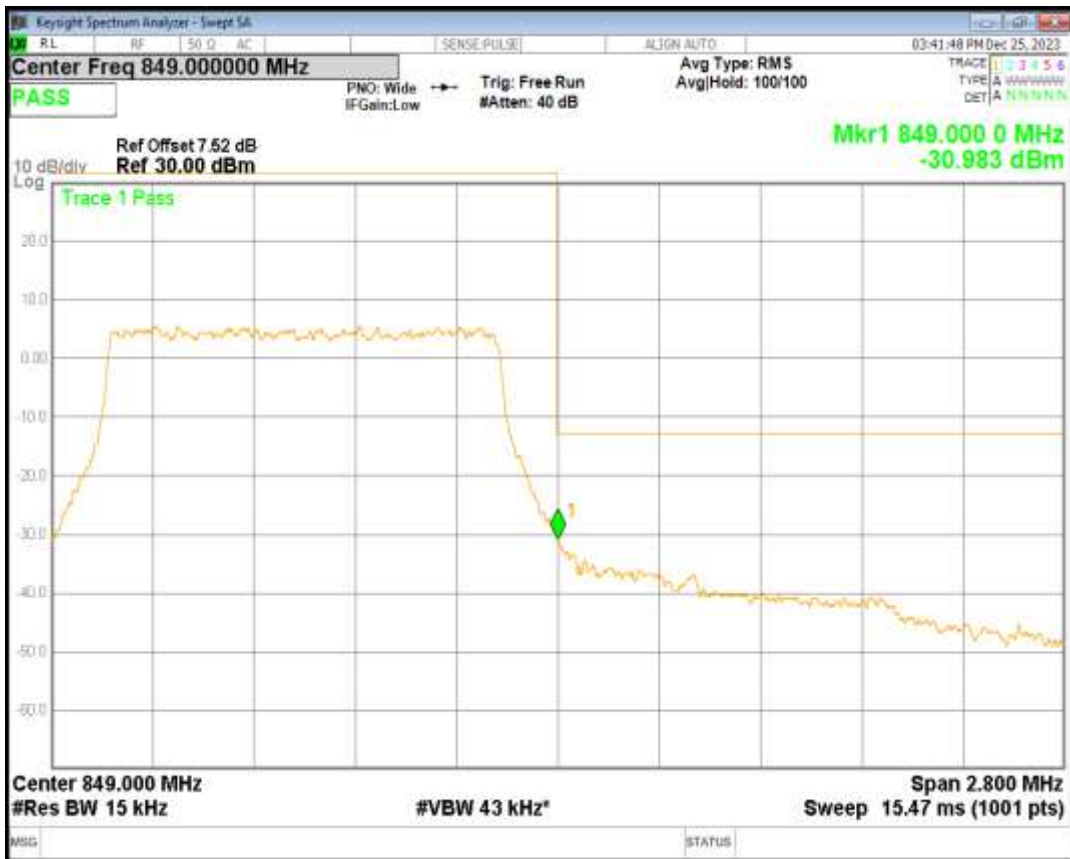
Band5 16QAM BW=1.4MHz Channel=20643 RB Size=6 Position=#0
