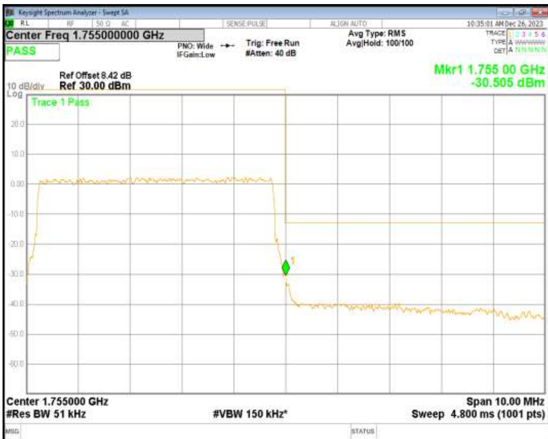
Band4 QPSK BW=10MHz Channel=20000 RB Size=50 Position=#0
